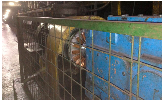
Figure 13. Application of permanent-magnet coupler in coal mining field.
