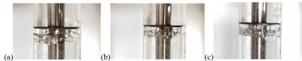
Figure 9. Drop size distribution of different reciprocating frequency: (a) 2 times/min, (b) 4 times/min, and (c) 6 times/min.
