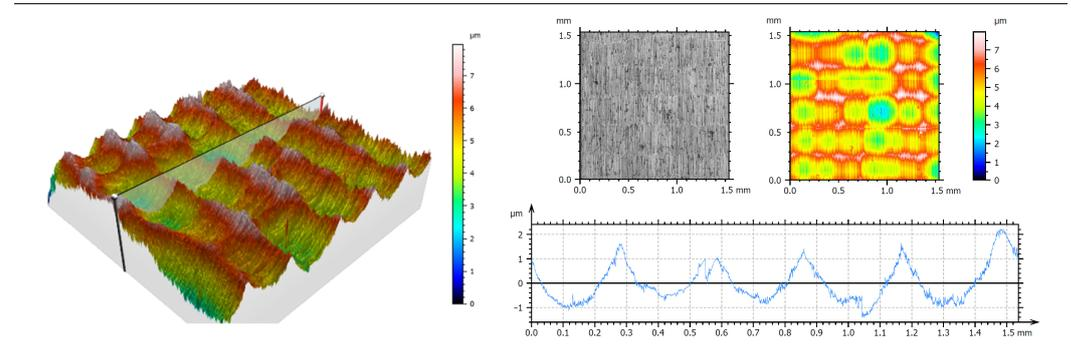
Three-dimensional view of surface texture and roughness profile at 30° Def 7.65
