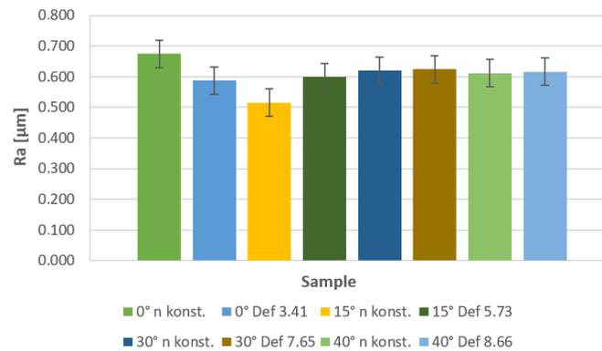
**Figure 9.** Comparison of roughness parameters Ra for concave parts of surfaces.
