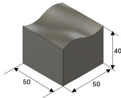
Figure 1. CAD model of sample.
