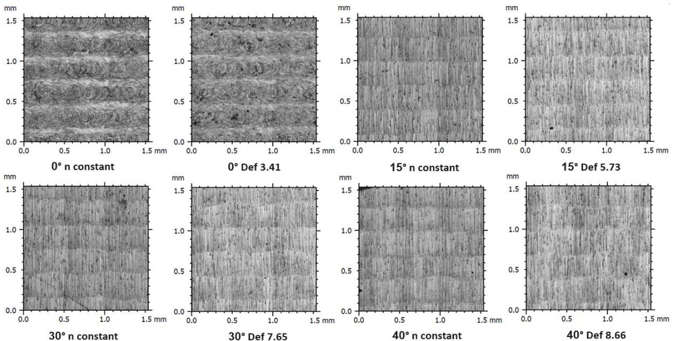
Figure 15. Two-dimensional topography of the convex parts of the surfaces according to the inclination of the tool.
