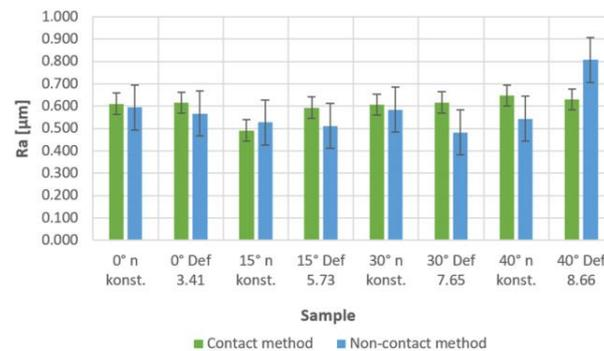
**Figure 19.** Values of the roughness parameters Ra for the convex part of the surface concerning the measurement method.
