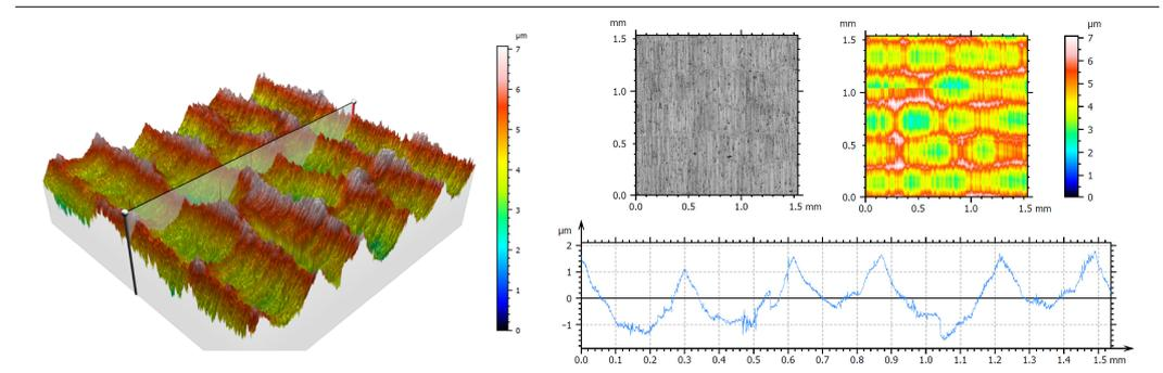
Three-dimensional view of surface texture and roughness profile at 40° n konstant
