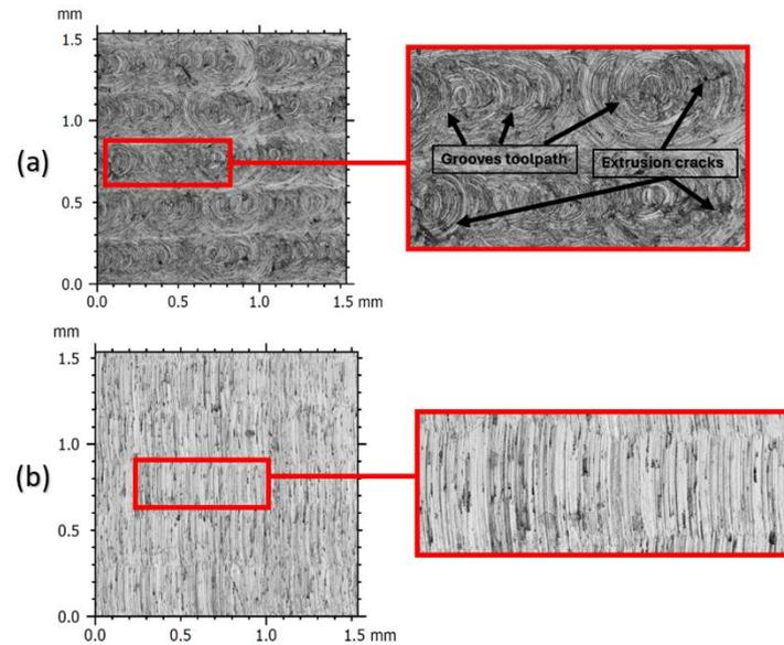
**Figure 18.** Two-dimensional topography comparison of produced samples, concave surface: (a) 0° n constant and (b) 15° n constant.
