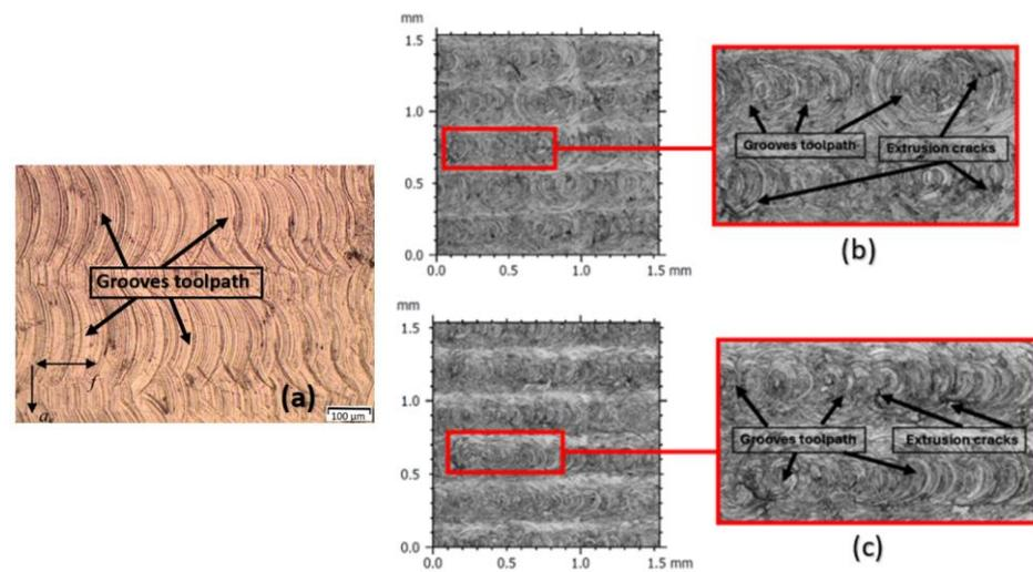
**Figure 23.** Surface morphology of linear strategy (a) 3-axis milling (b) 5-axis milling, concave surface  $0^\circ$  n constant (c) 5-axis milling, convex surface  $0^\circ$  n constant.
