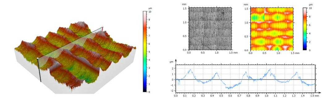
Three-dimensional view of surface texture and roughness profile at 30° n konstant
