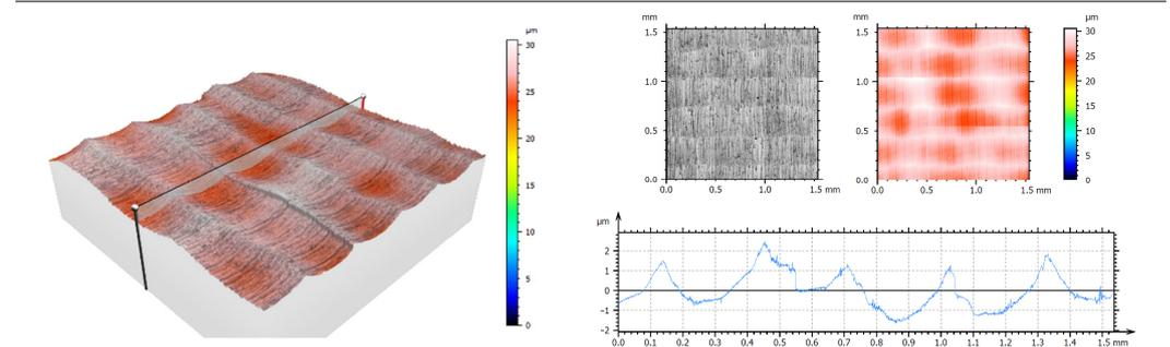
Three-dimensional view of surface texture and roughness profile at 30° Def 7.65
