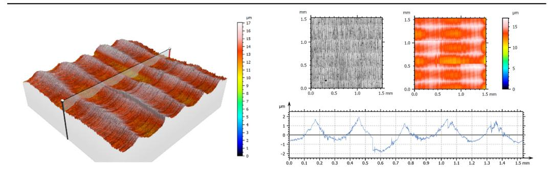
Three-dimensional view of surface texture and roughness profile at 15° Def 5.73
