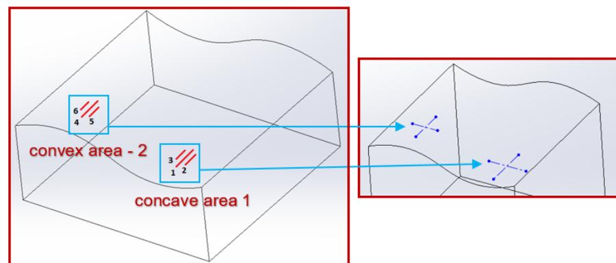
**Figure 6.** Marked measurement points on the convex and concave part of the sample surface for measuring the surface roughness.
