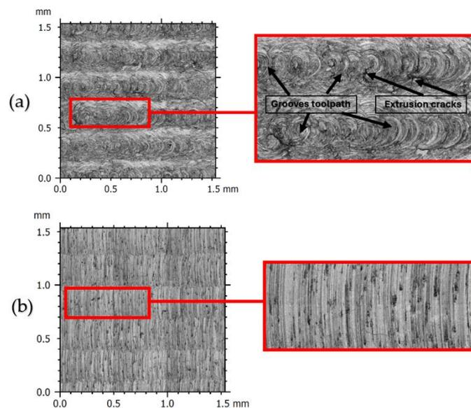
**Figure 17.** Two-dimensional topography comparison of produced samples, convex surface: (a)  $0^\circ$  n constant and (b)  $15^\circ$  n constant.
