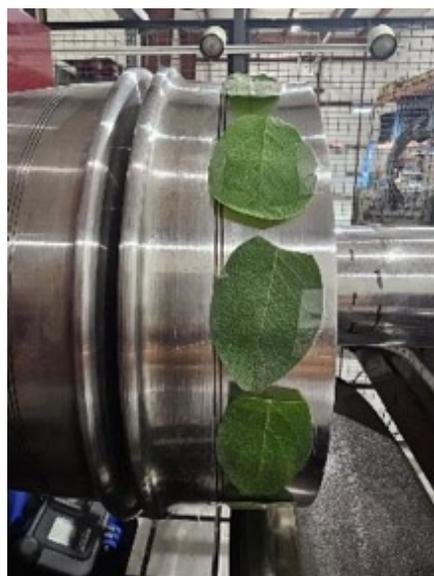
**Figure 6.** Application of leaves to a clean wheel surface with adhesive tapes on the edges, away from the running surfaces.
