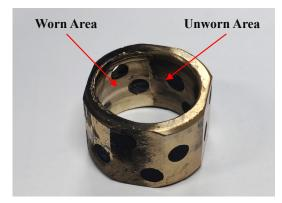
Figure 11. The worn bearing.
