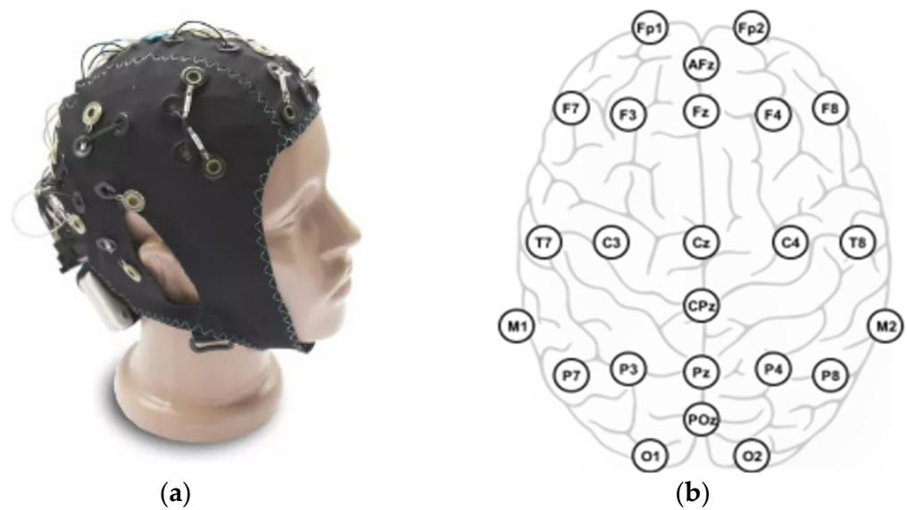
**Figure 5.** (a) Electroencephalogram (EEG) gel-based cap and (b) view of the localization of the electrodes on the scalp by the software SMARTING.
