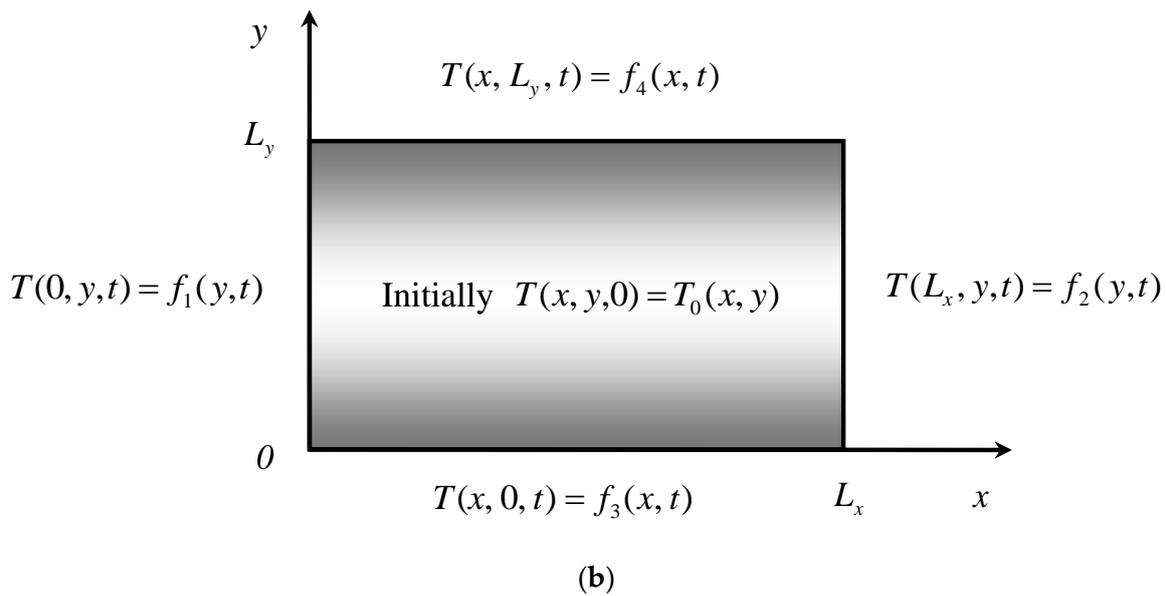
**Figure 1.** The 2D heat conduction in a rectangular cross-section of an infinite bar with general Dirichlet boundary conditions. (a) An infinite bar with a rectangular cross-section. (b) The 2D heat transfer system in a rectangular region (cross-section).
