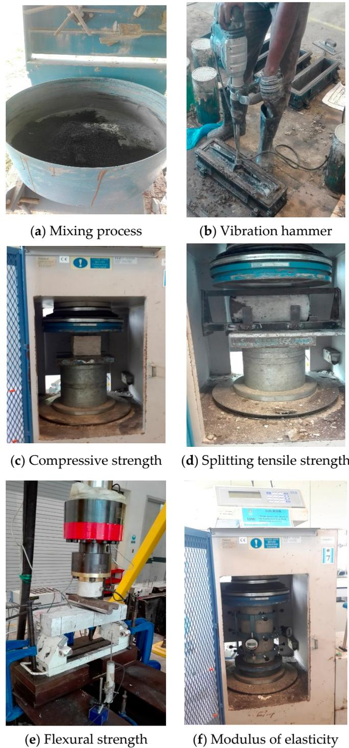
**Figure 3.** Experimental setup.
