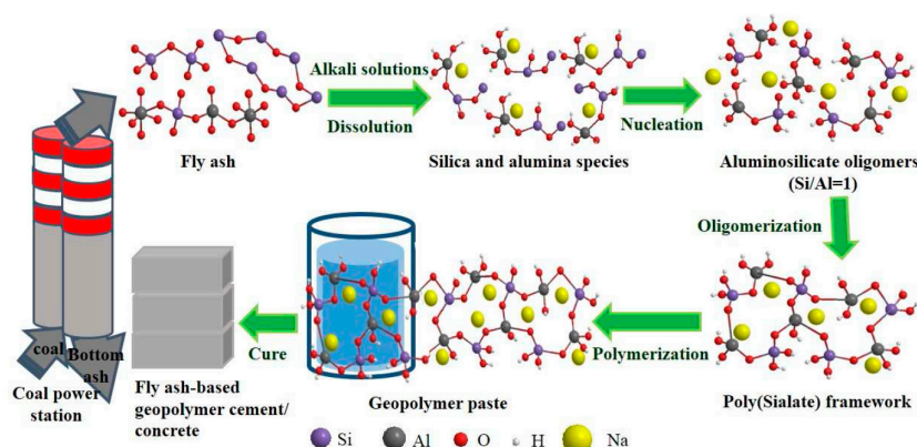
Figure 2. Processes of geopolymerization from FA [7] (Reproduced with permission from Journal of Cleaner Production; published by Elsevier, 2016).
