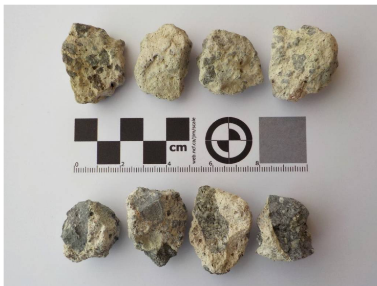
Figure 3. (Top) Plant-recycled gravel showing fragments entirely composed of mortar (sand and cement paste). (Bottom) Laboratory-recycled gravel with aggregates composed of rock with adhered mortar.
