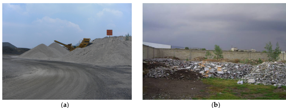
Figure 1. (a) Mounds of recycled gravel at the Concretos Reciclados S.A. plant; (b) a landfill containing construction and demolition waste (CDW) where the demolished concrete was collected.
