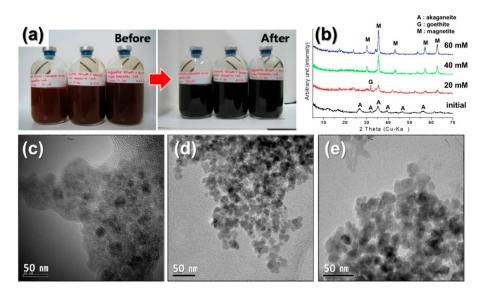
**Figure 3.** Microbial synthesis of magnetite nanoparticles at different concentrations of magnetite precursors: (a) Color changes by the mineral phase transition, (b) XRD patterns, TEM images of magnetite formed by Haejae-2 with different concentrations of akaganeite [(c) 20 mM, (d) 40 mM, (e) 60 mM].
