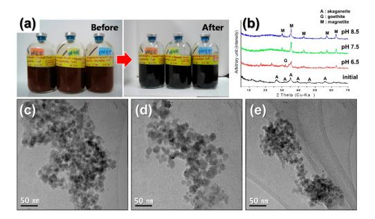
**Figure 4.** Microbial synthesis of magnetite nanoparticles at different pHs of medium: (**a**) Color changes by the mineral phase transition, (**b**) XRD patterns, TEM images of magnetite formed by Haejae-2 at different pH values of media at (**c**) pH = 6.5, (**d**) pH = 7.5, (**e**) pH = 8.5.
