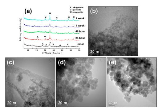
**Figure 5.** Microbial synthesis of magnetite nanoparticles at different incubation time: (**a**) XRD patterns, TEM images of magnetite formed by Haejae-2 at different incubation time [(**b**) 24-h, (**c**) 48-h, (**d**) 1-week, (**e**) 2-week].
