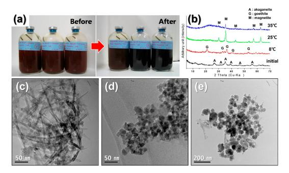
**Figure 2.** Microbial synthesis of magnetite nanoparticles at different incubation temperatures: (a) Color change followed by the mineral phase transition, (b) X-ray diffraction (XRD) patterns, TEM images of magnetite formed by Haejae-2 at different incubation temperatures at (c) 8 °C, (d) 25 °C, (e) 35 °C.
