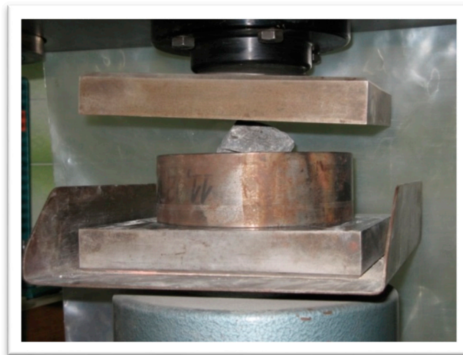
Figure 2. Single axial compression of individual particle between two plates in the hydraulic piston-die press, (manufactured by Tony Technik; Institute of Ceramics and Building Materials, Glass and Building Materials Division in Cracow, Poland).
