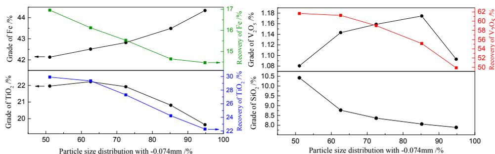
Figure 5. The effect of grinding fineness on low-intensity magnetic separation.
