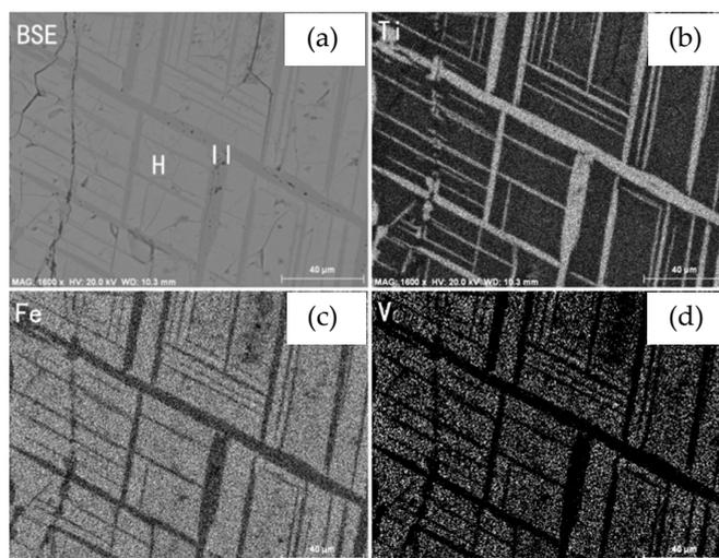
**Figure 1.** SEM images of vanadium-titanium magnetite replaced by martite: (a) Back-scattered electron image; (b) Ti element mapping; (c) Fe element mapping; (d) V element mapping.
