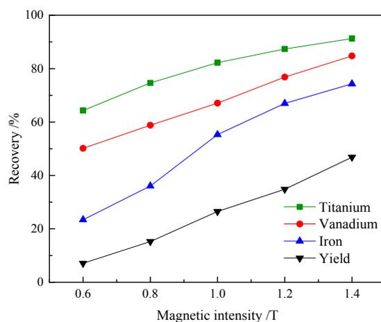
Figure 4. The effect of magnetic intensity on the pre-discarding tailing.
