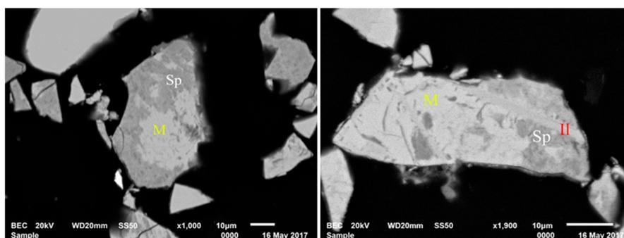
Figure 7. SEM images of the vanadium-titanium magnetite concentrate.
