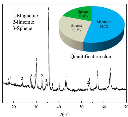
Figure 6. XRD patterns of the vanadium-titanium magnetite concentrate.
