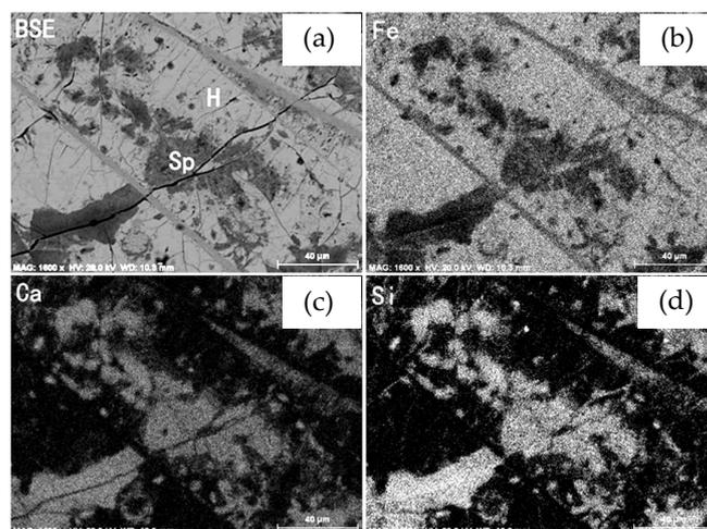
**Figure 2.** SEM images of vanadium-titanium magnetite replaced by sphene: (a) Back-scattered electron image; (b) Fe element mapping; (c) Ca element mapping; (d) Si element mapping.
