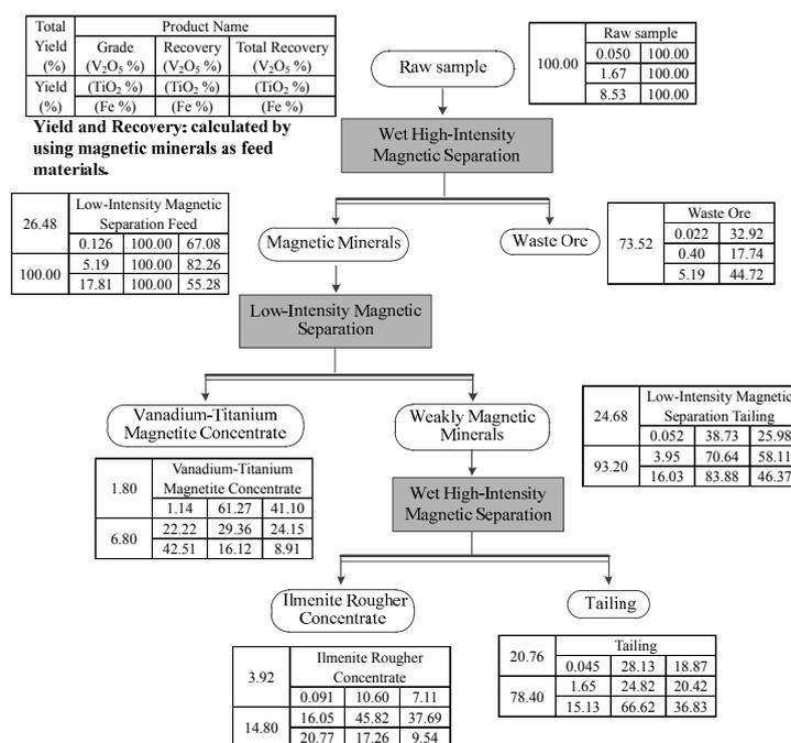
**Figure 8.** Flow-sheet for the pre-concentration of low-grade vanadium-titanium magnetite ore.
