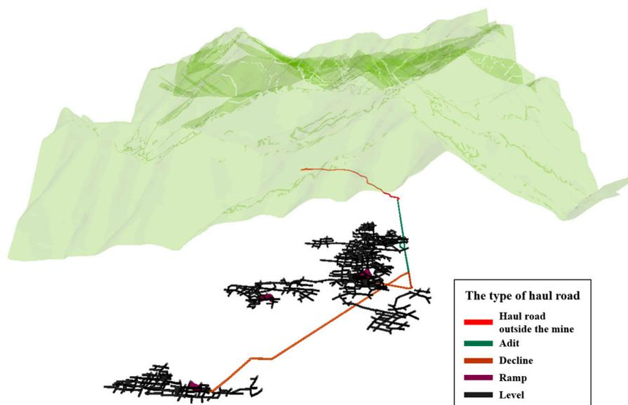
**Figure 3.** Three-dimensional view of haul roads constructed in the underground mine. Haul roads consist of an adit, declines, ramps, levels, and a haul road outside the mine.
