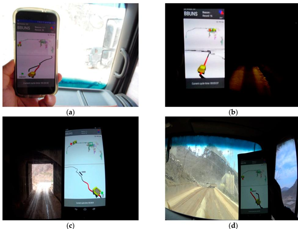
**Figure 9.** Results of testing the BBUNS application during the haulage operation when (a) leaving the crushing plant, (b) driving toward the 540 ML workplace, (c) passing by the portal of the underground mine, and (d) returning to the crushing plant.
