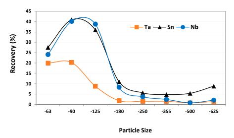
**Figure 18.** Average recovery by particle size during separation by a Knelson concentrator. Recoveries calculated from PXRF results.
