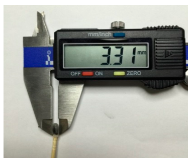
Figure 2. Diameter measurement of the ore core.
