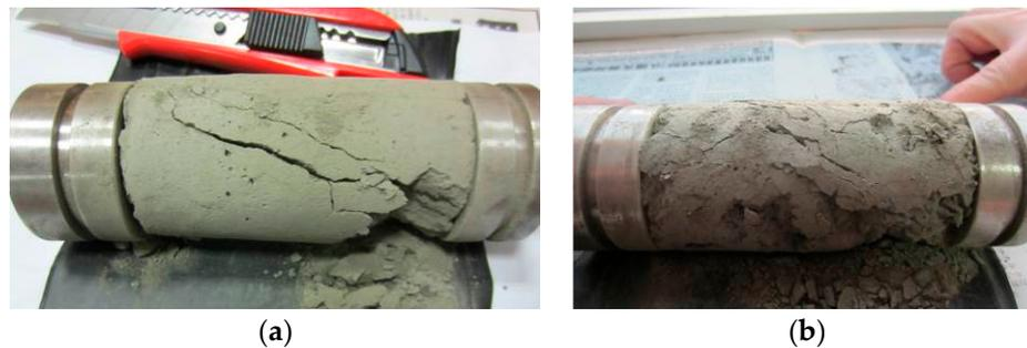
**Figure 11.** Specimen form after the failure of the mixed disposal with different waste rock contents. (a) Waste rock content of 10%; and (b) waste rock content of 50%.
