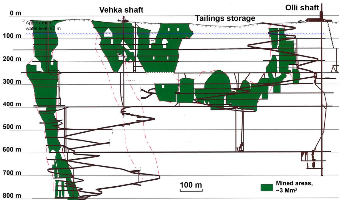
**Figure 1.** Schematic cross section of Kotalahti Mine showing Vehkankuilu and Ollinkuilu shafts. The green areas show the excavated parts of the mine, the red lines outline the ore body in the mafic and ultramafic complex. The two shafts, Vehkankuilu and Ollinkuilu, are situated approximately 1 km apart. Modified from [9,10]. Depths are given as below ground level. The water level is indicated with a blue line.
