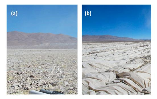
**Figure 3.** Run-of-mine dump bioleach at Escondida, Chile showing (**a**) surface with irrigation lines and (**b**) covers to retain heat and moisture. Photographs by D.W. Shiers, reproduced with permission.
