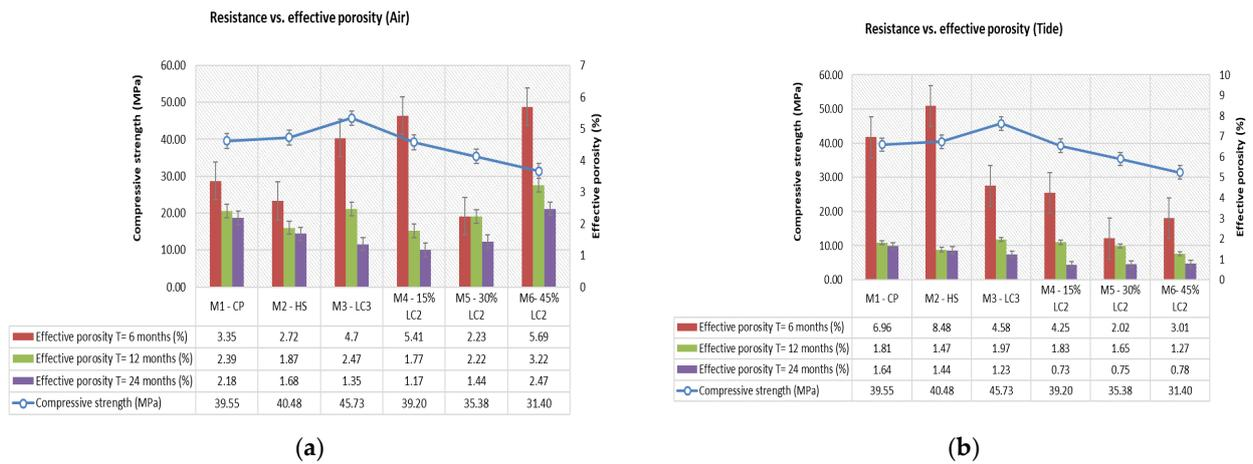
Figure 6. Effective porosity 6–24 months exposure; (a) Air Zone; (b) Tidal Zone.
