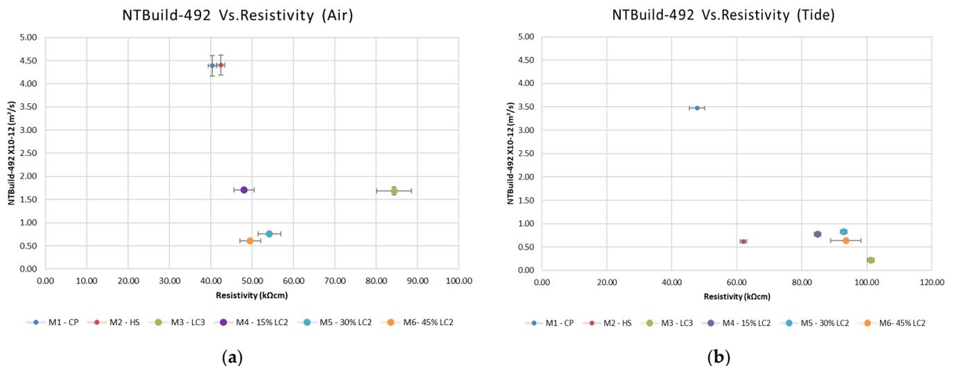
Figure 11. Chloride migration Vs. resistivity; (a) Air Zone; (b) Tidal Zone.
