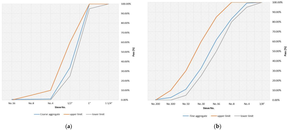
**Figure 1.** Particle size distributions of the aggregates, (a) coarse aggregate, (b) fine aggregate.
