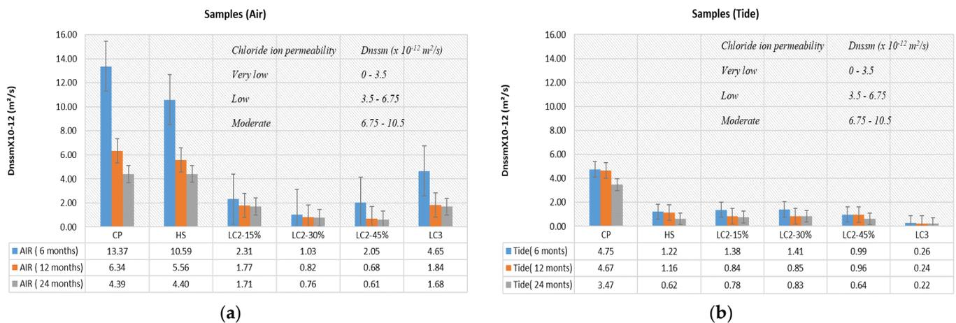
Figure 10. Chloride migration values recorded; (a) Air Zone; (b) Tidal Zone.
