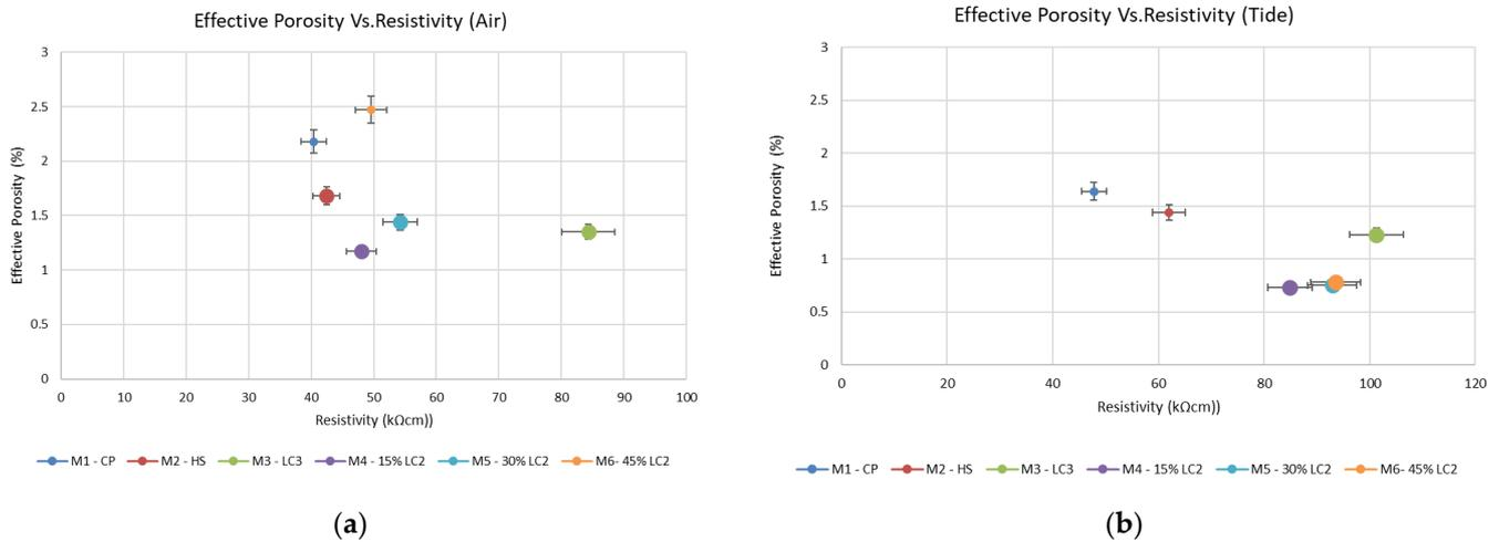
Figure 8. Effective porosity Vs. electrical resistivity; (a) Air Zone; (b) Tidal Zone.
