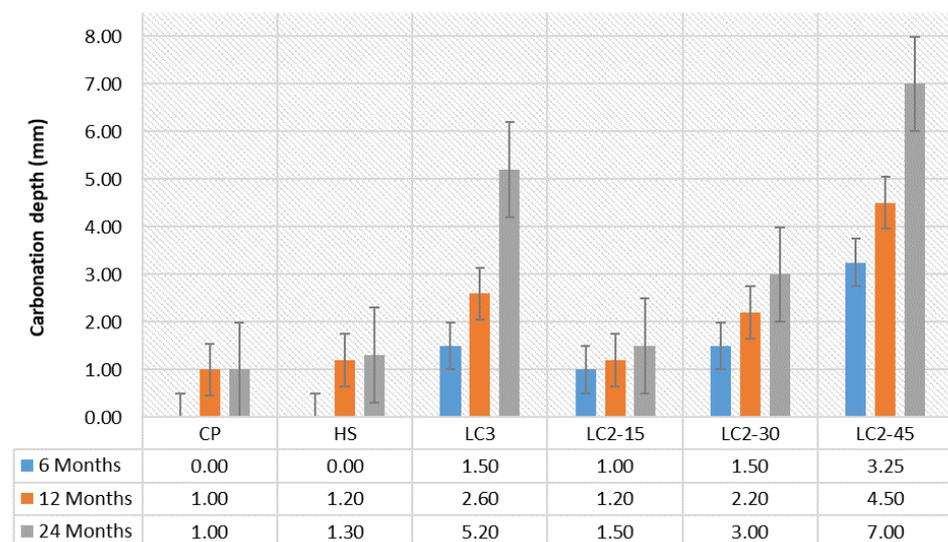
**Figure 12.** Carbonation in Air zone concrete.
