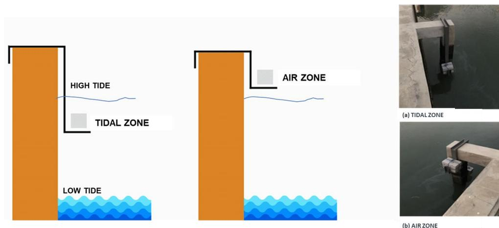
Figure 4. Exposure zones of the elements, (a) Tidal zone, (b) Air zone.
