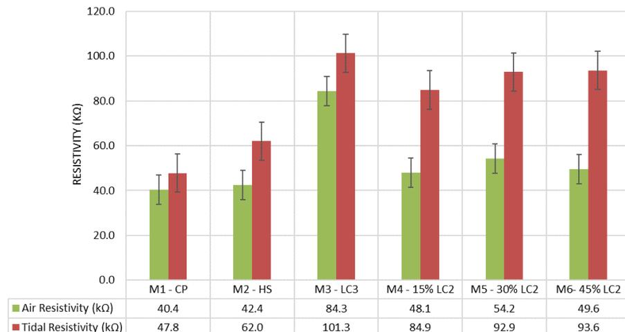
Figure 7. Electrical resistivity after 24 months.
