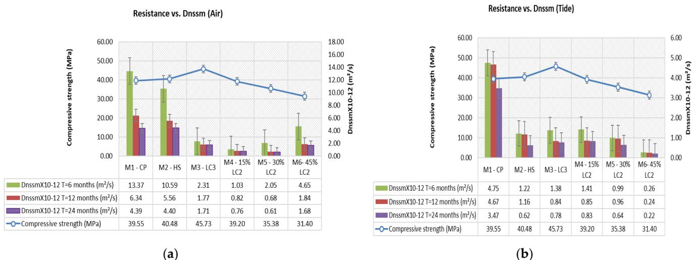
Figure 9. Compressive strength vs. Dnssm ratio (a) Air zone; (b) Tidal zone.
