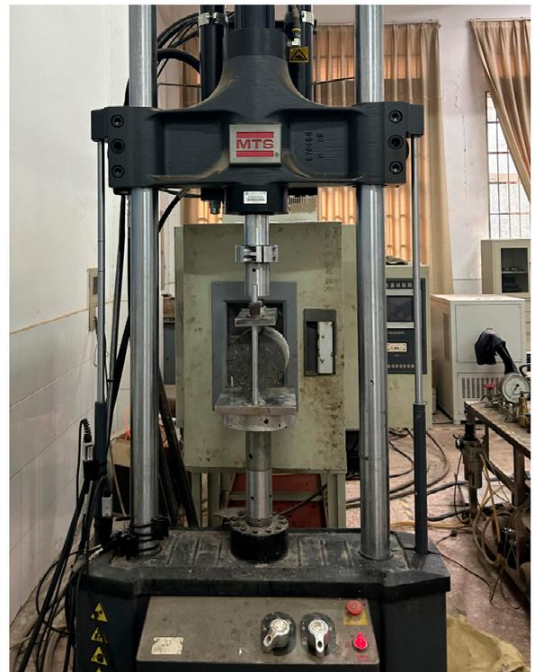
(b) Splitting strength test
