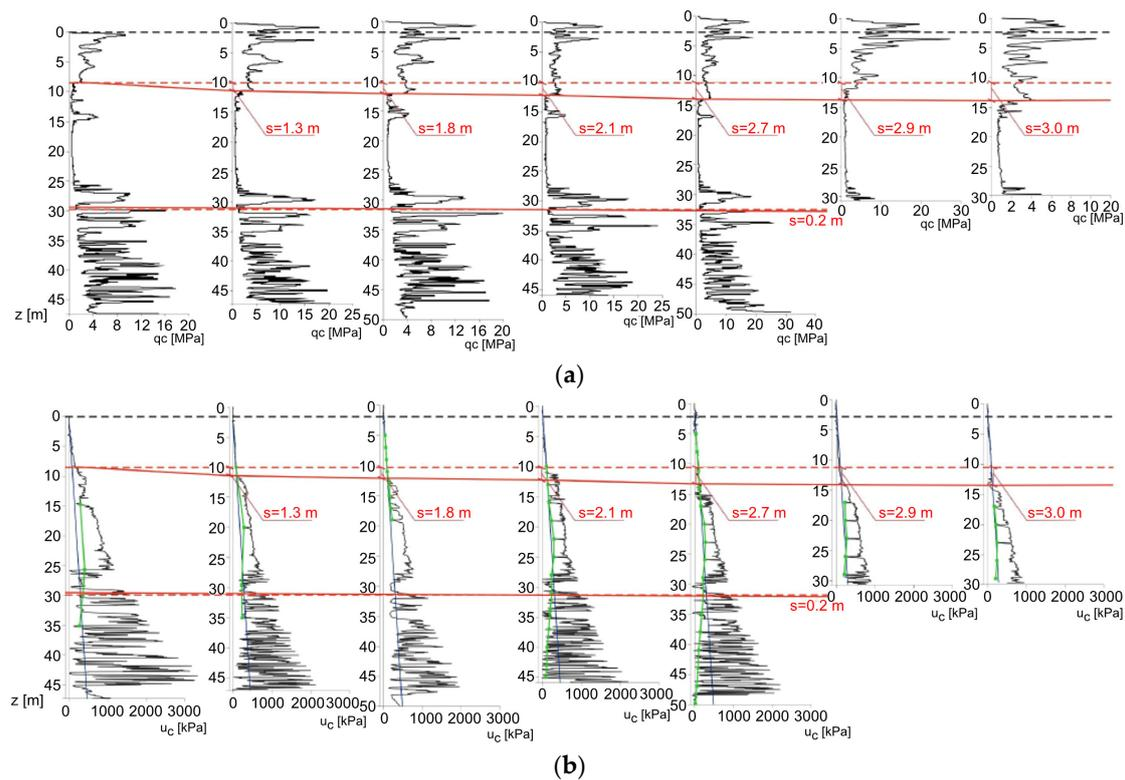
**Figure 8.** (a) The settlements assessed by the graphical direct method at point 1+000 over a period of more than 2 years:  $q_c$  curves; (b) dissipation curves  $u_c$ . The dashed line corresponds to a value of  $s = 0.0$  m, and the distance between the dashed line and the solid line represents the value of  $s$  [m].
