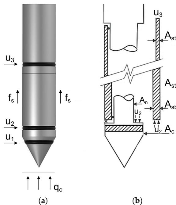
**Figure 4.** (a) Cone used for penetration test, author’s own drawing; (b) the influence of pore water pressure on measured penetration parameters [8], where  $A_n, A_{st}, A_{sb}$ —cross-sectional areas.
