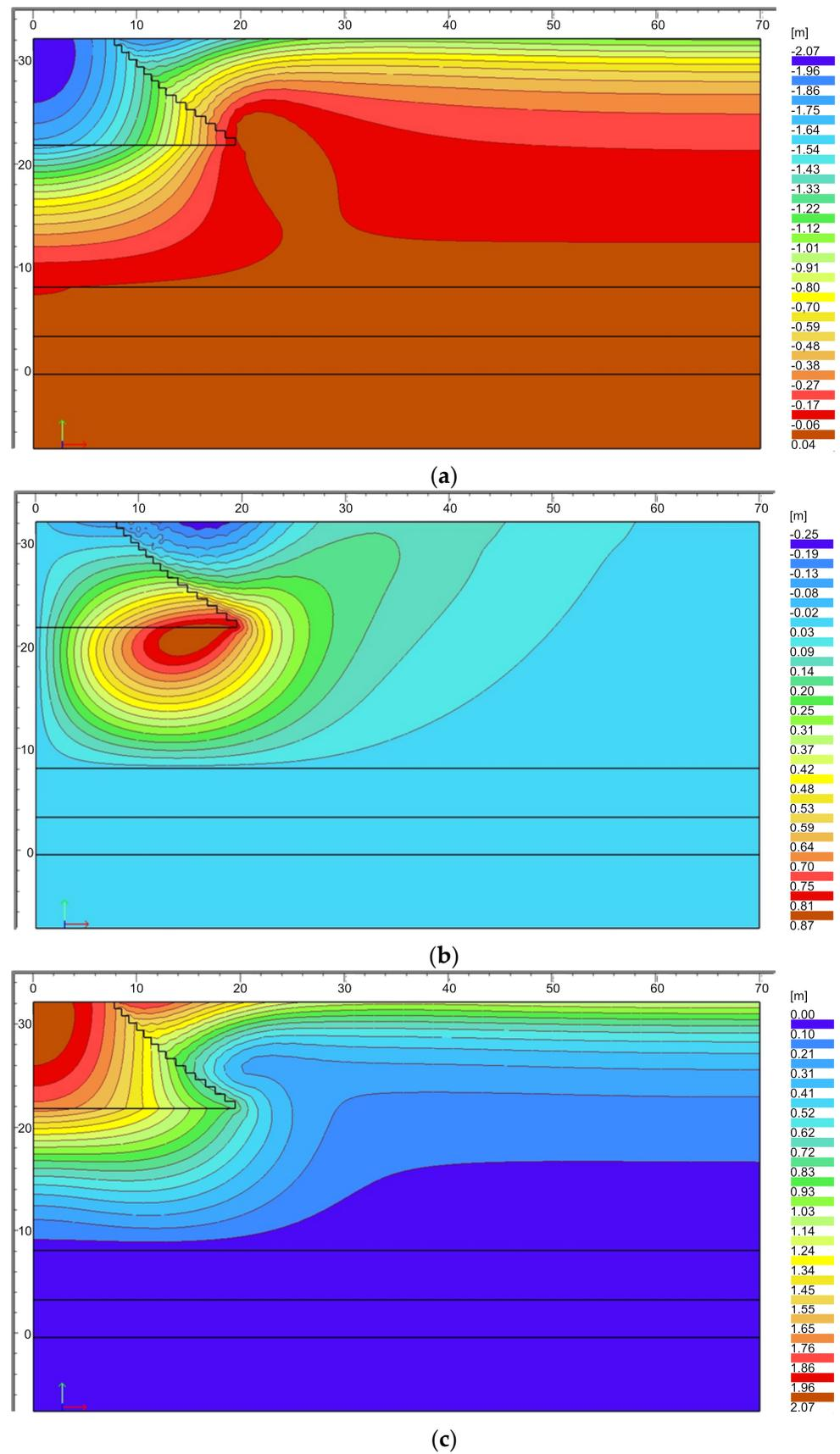
Figure 12. Displacements in Stage II: (a) vertical; (b) horizontal; (c) total.
