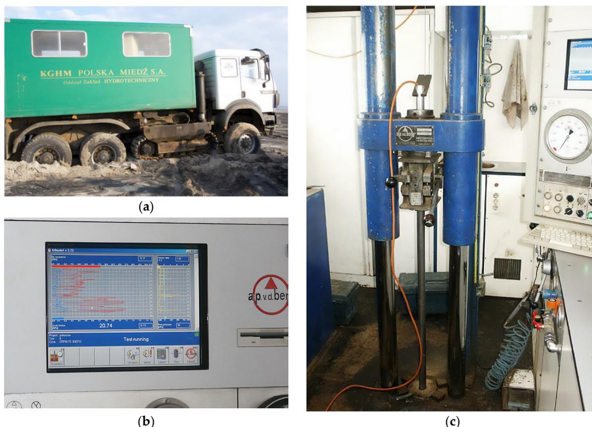
**Figure 5.** (a) Hyson 200 kN track-truck type by a.p. van den Berg company (Heerenveen, Netherlands); (b) touch screen by a.p. van den Berg company (Heerenveen, Netherlands); (c) interior of the Hyson, photo: KGHM Polska Miedź (Lubin, Poland).
