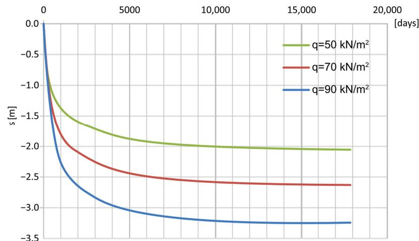
Figure 15. Settlements after the consolidation.
