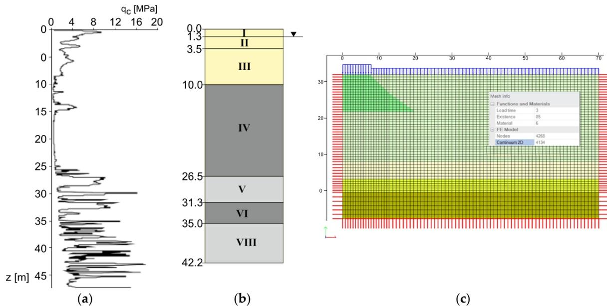
Figure 10. Point 1+000: (a) cone resistance distribution  $q_c$ ; (b) calculation scheme based on  $q_c$ ; (c) generated mesh of elements.
