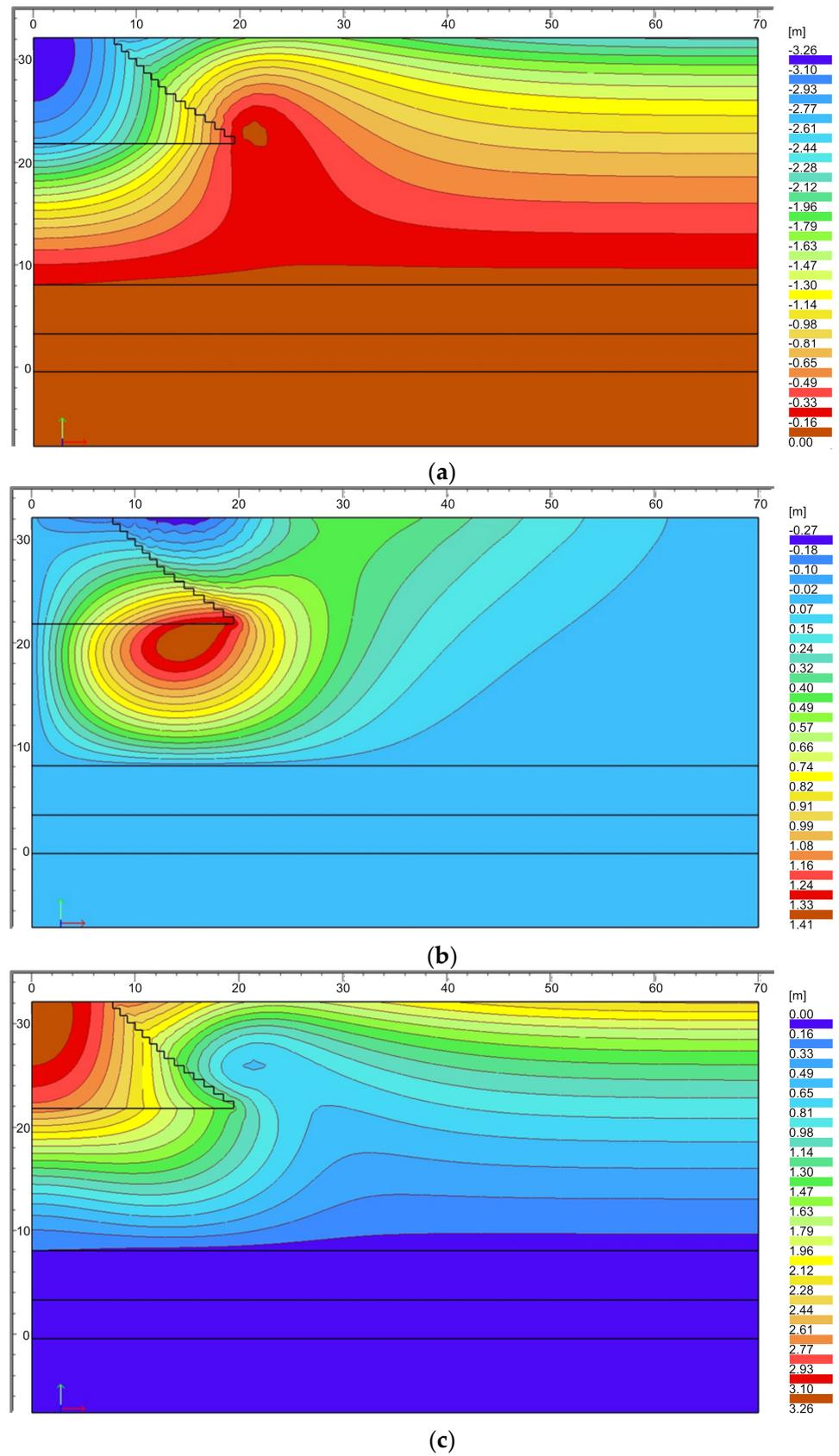
Figure 13. Displacements in Stage III: (a) vertical; (b) horizontal; (c) total.
