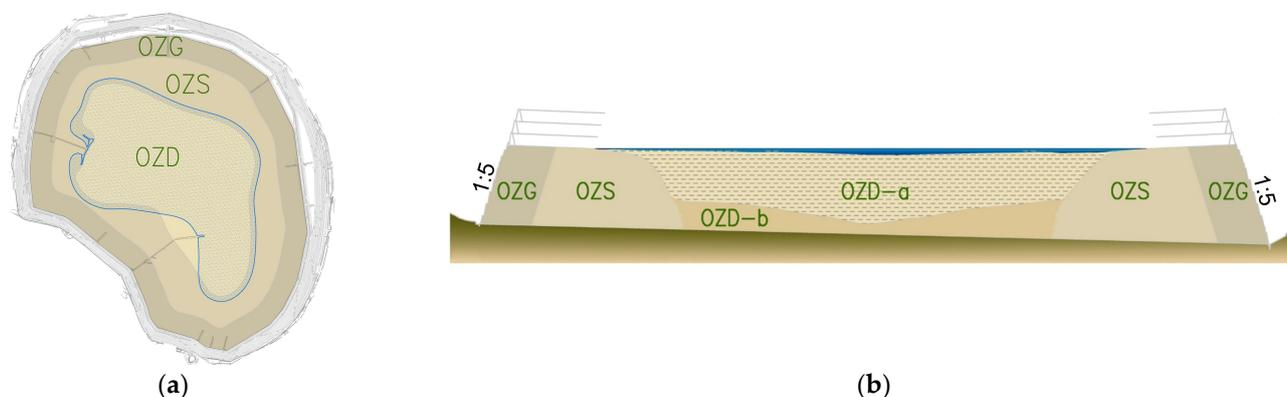
**Figure 3.** (a) Generalized grain size distribution of tailings deposited in the TSF; (b) an example cross-section through the storage facility, where OZG—coarse tailings used for dam construction, OZS—coarse tailings with some amount of fines, OZD—fine tailings deposited in the pond: OZD-a—fine tailings in liquid state, and OZD-b—consolidated fine tailings.
