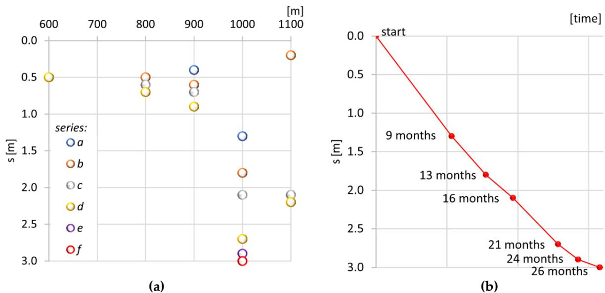
**Figure 7.** Graphical interpretation of settlements determined by the direct method: (a) points 0+600–1+100; (b) point 1+000.
