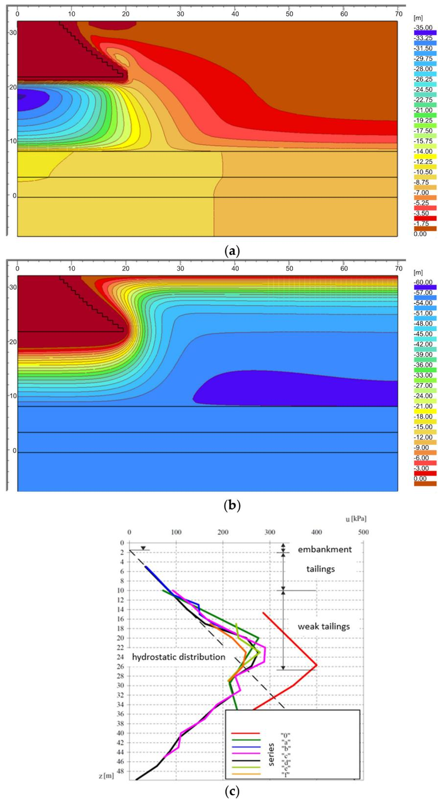
**Figure 14.** Pore water pressure excess: (a) at the beginning of Stage I; (b) at the end of Stage I; (c) actual distributions of pore water pressure (dissipation tests). The dashed line illustrates the hydrostatic pressure distribution.
