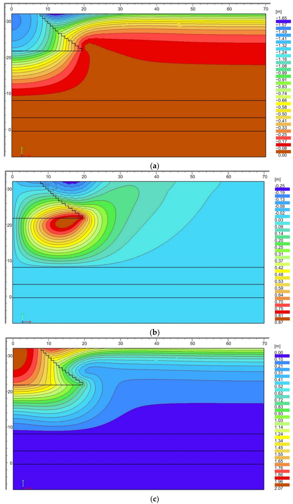
Figure 11. Displacements in Stage I: (a) vertical; (b) horizontal; (c) total.
