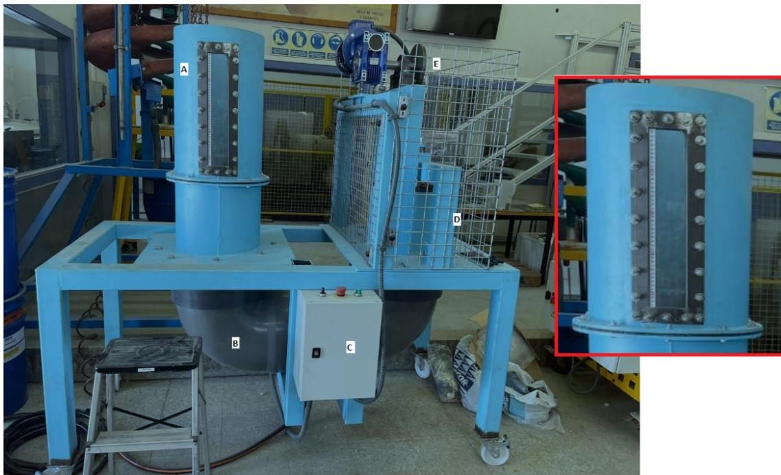
**Figure 4.** Image of the jig equipment used in the experiments: (A) jig chamber (enlarged), (B) water passage duct, (C) electric panel, (D) pump chamber, and (E) motor.
