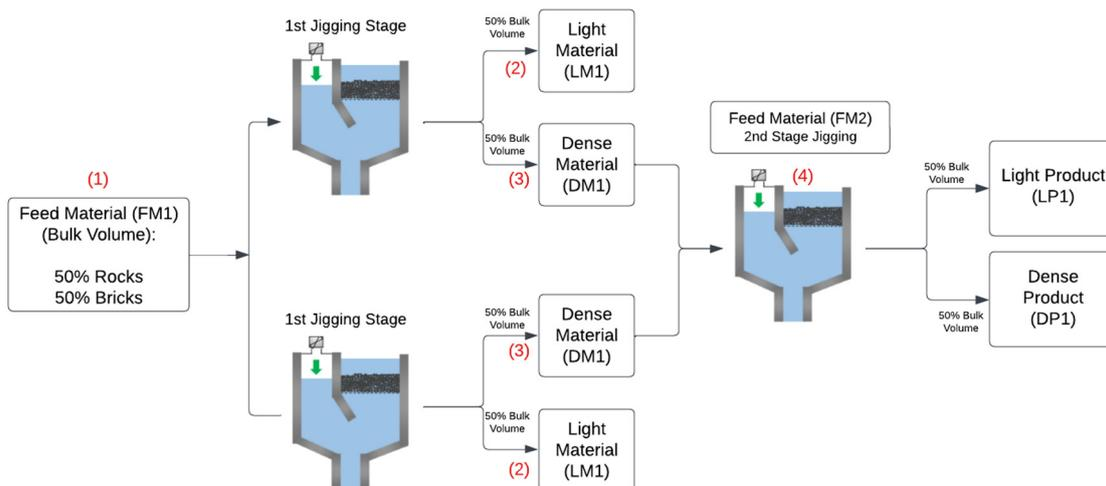
**Figure 5.** The flowchart of the two-stage jigging process made to concentrate the binary mixture of rocks and bricks.
