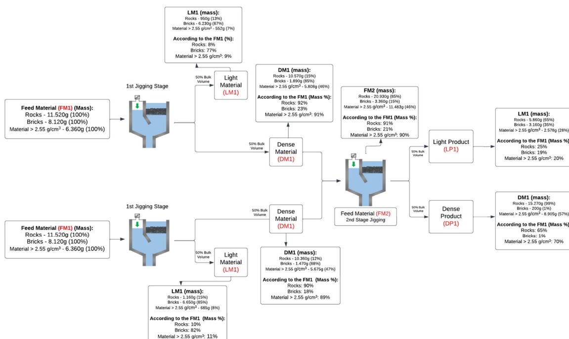
**Figure 9.** The flowchart of the jig tests and mass balance of the binary test.
