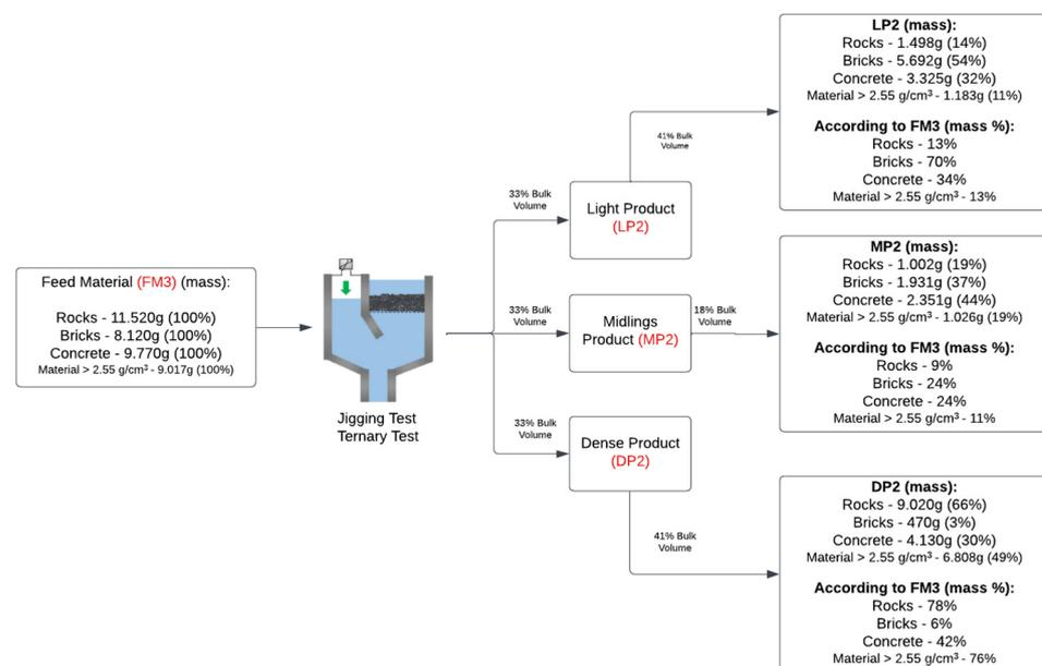
**Figure 10.** The flowchart of the jig tests and mass balance of the ternary test.
