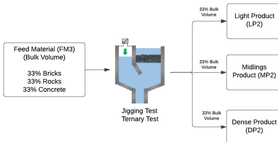
**Figure 6.** The flowchart of the jigging process made to concentrate the ternary mixture of rocks, concrete, and bricks.
