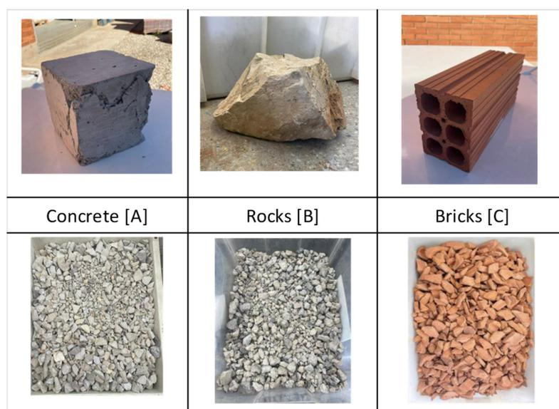
**Figure 3.** (A) Concrete before and after the preparation, (B) rocks from old houses before and after the preparation, and (C) bricks before and after the preparation.
