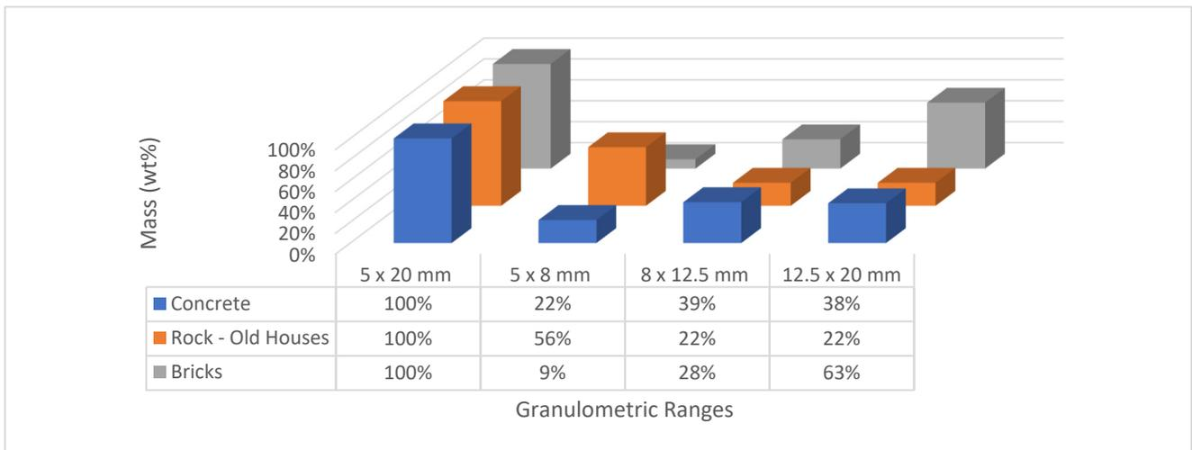
Figure 8. Granulometric distribution of the rocks, concrete, and bricks with 5 × 20 mm range.
