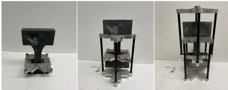
**Figure 9.** Compression to tensile load converter assembly.
