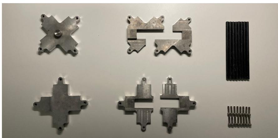
**Figure 6.** Compression to tensile load converter components.
