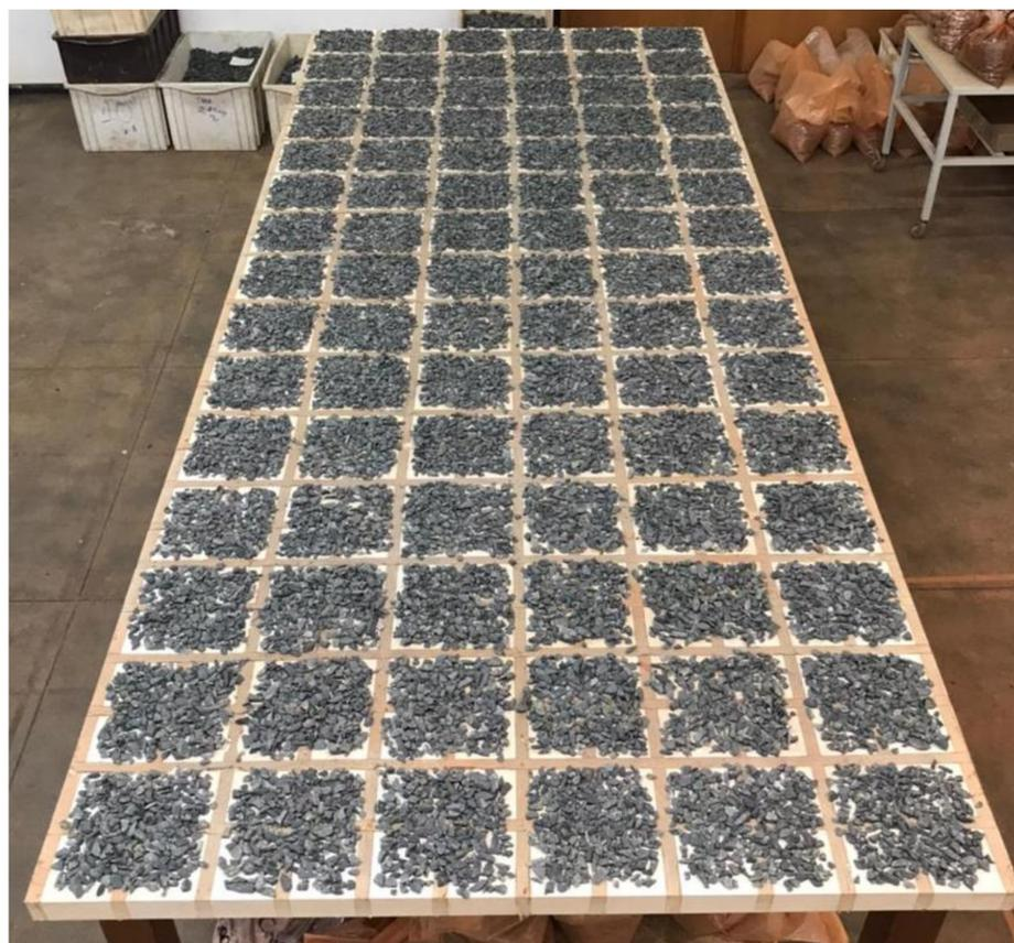
**Figure 1.** Material spread on the grid for the HT, size fraction –12.7 mm +6.35 mm.
