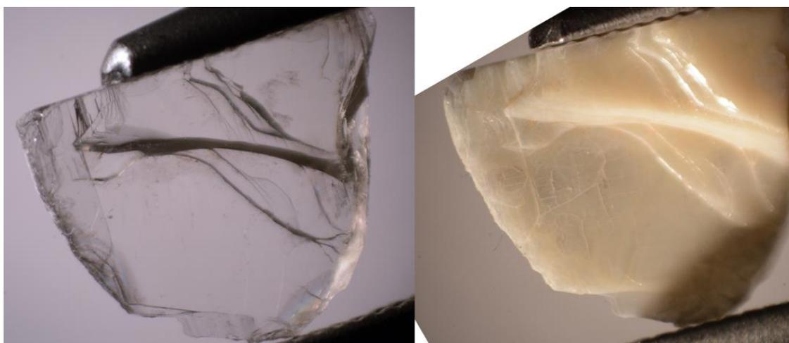
**Figure 5.** The colorless diaspore fragment (sample 97003) before heating (**left**), transformed to whitish corundum with tiny micro-fissures after dehydration (**right**). Image width 10 mm.
