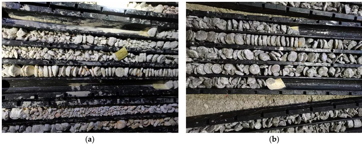
**Figure 1.** Core disking in a deep mine in China: (a) Mining depth of 950 m; (b) Mining depth of 1050 m.
