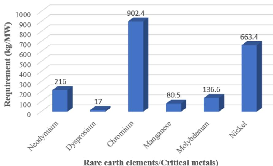
Figure 3. Rare earth and special metal demand for wind turbine technology estimated in kg/MW [30,31].
