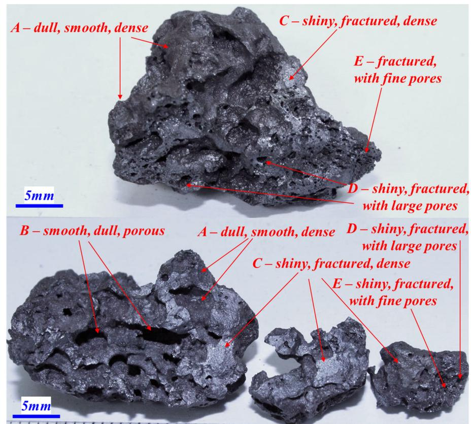
**Figure 2.** Example of Macro-Types A~E on industrial sinter products.
