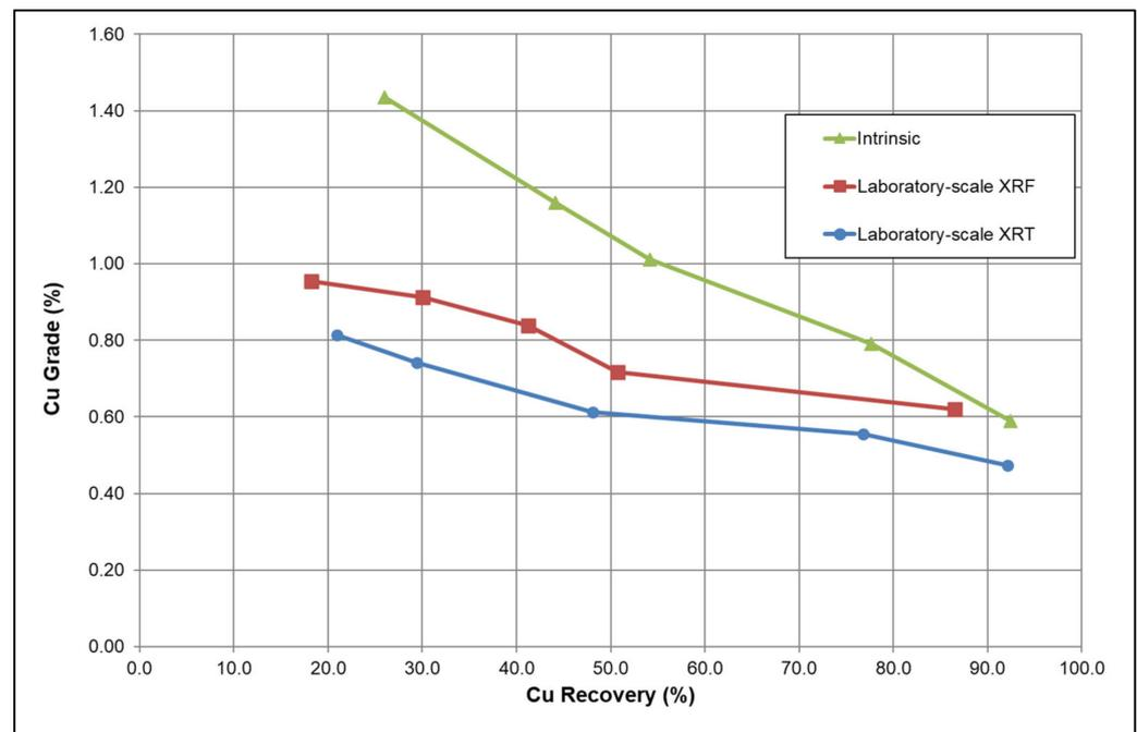
**Figure 8.** Cumulative grade-recovery curves for the intrinsic and laboratory (ideal) sensor tests.
