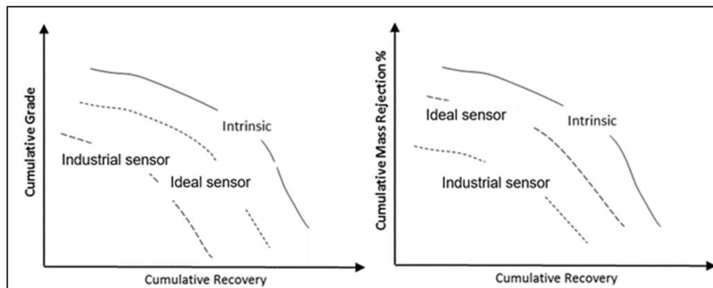
**Figure 3.** Examples of cumulative grade, recovery and mass rejection curves comparing the intrinsic, ideal sensor and industrial sensor sortability tests.
