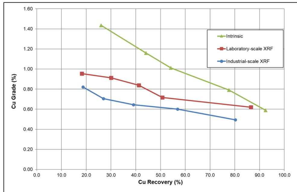
**Figure 9.** Cumulative grade-recovery and mass rejection curves for the intrinsic, ideal and industrial sensor tests.
