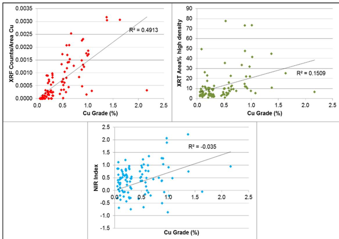
Figure 7. XRF, XRT and NIR sensor response curves.
