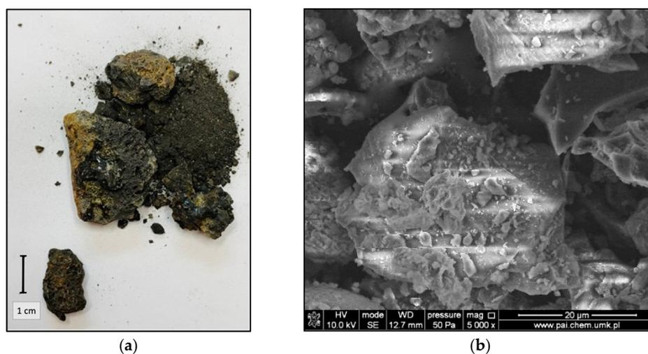
**Figure 1.** Overview photo of the Blast Furnace Slag used in study (a). Scanning electron microscopy (SEM) image at  $5000\times$  magnification of the Blast Furnace Slag (b).
