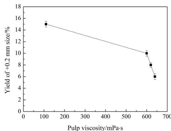
**Figure 4.** The relationship between pulp viscosity and the 0.2 mm size fraction yield.
