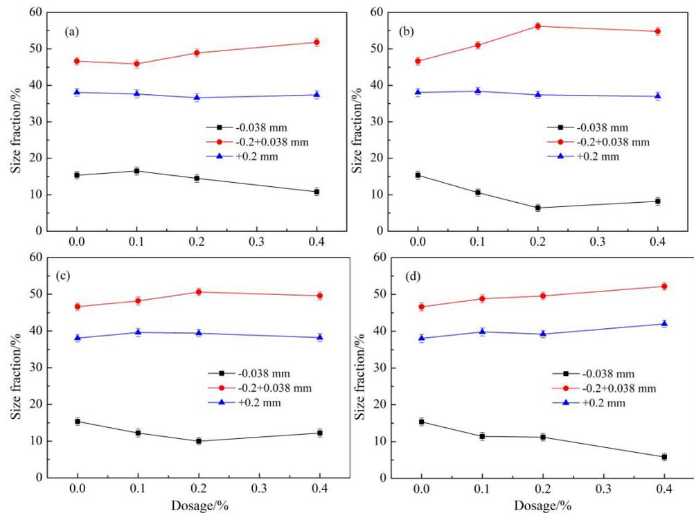
**Figure 2.** The effects of polyacrylamide molecular weight on the grinding product size with (a) PAM300, (b) PAM500, (c) PAM800 and (d) PAM1200.
