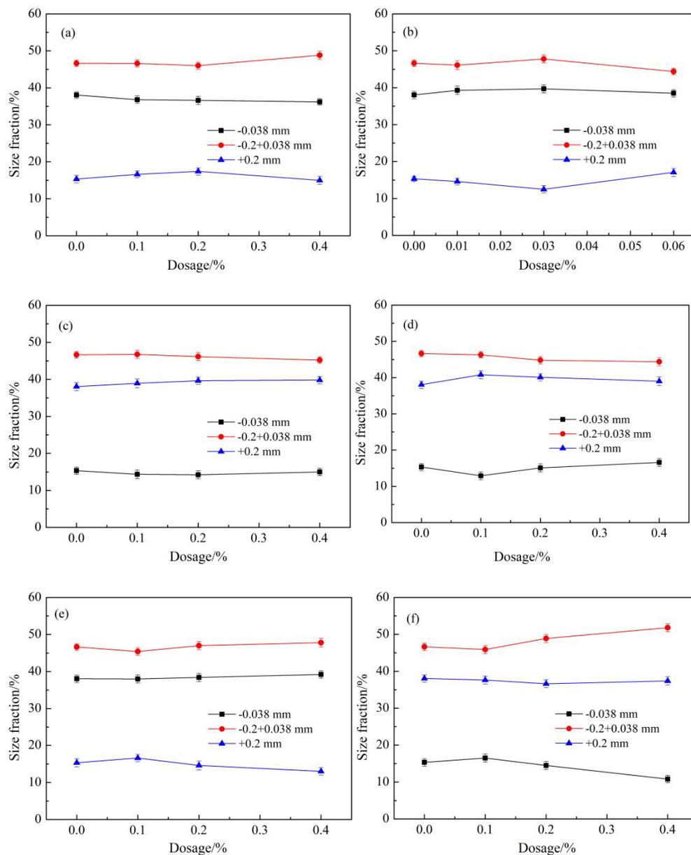
**Figure 1.** The plots of the yields of product size fractions against the dosage of (a) sodium hexametaphosphate, (b) triethanolamine, (c) ferric sulphate, (d) aluminum chloride, (e) polyaluminum chloride and (f) PAM300.
