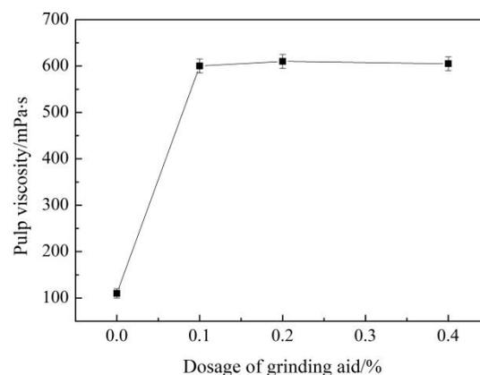
**Figure 3.** The relationship between pulp viscosity and grinding aid dosage.
