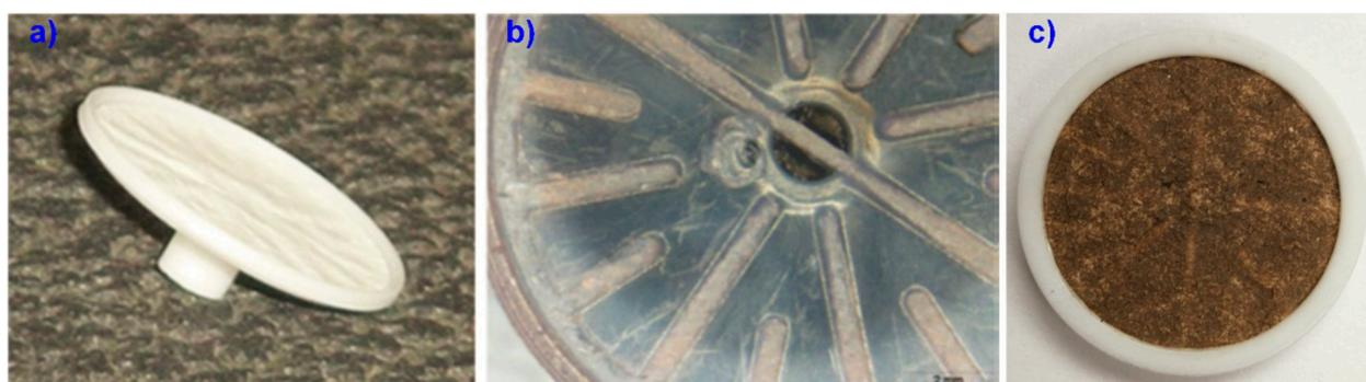
**Figure 4.** Examples of: (a) a clean PDM filter holder; (b) backside of a PDM filter holder showing structural bars; and (c) a PDM filter with a nonuniform particle deposit affected by the filter holder [64]. Reprinted by permission of Taylor & Francis Ltd.
