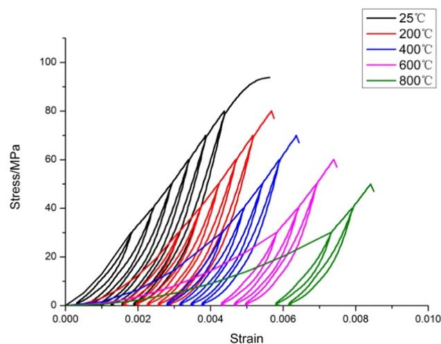
**Figure 4.** Stress–strain curves of sandstone after different high temperatures.
