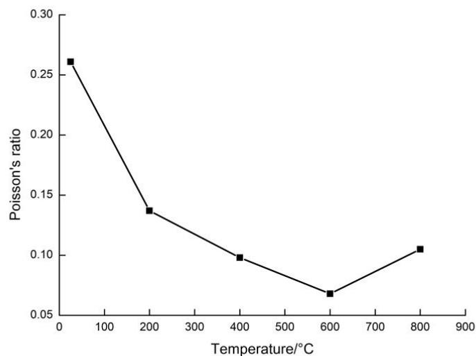
**Figure 7.** The relationship between Poisson's ratio and temperature for sandstone.
