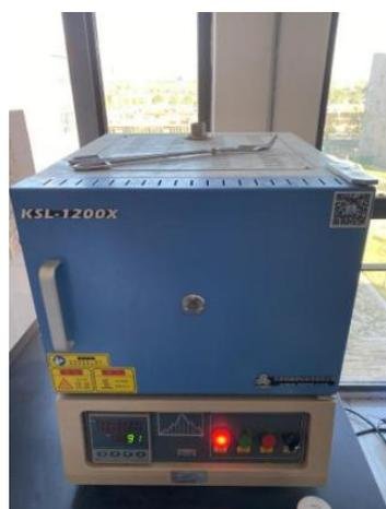
**Figure 1.** Box-type high-temperature fritting furnace.
