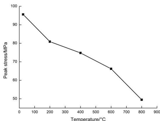
**Figure 5.** Peak stress in sandstone as a function of temperature.
