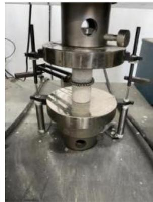
**Figure 3.** Single-axis cyclic loading and unloading tester.
