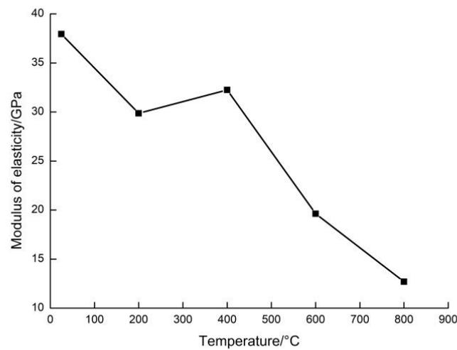
**Figure 6.** Modulus of elasticity of sandstone as a function of temperature.
