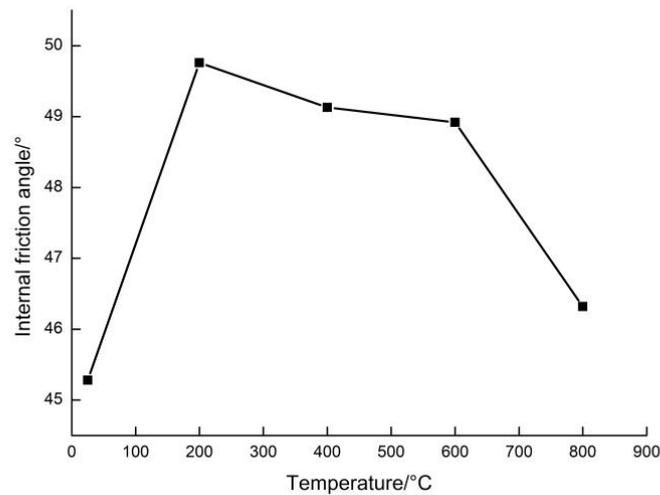
**Figure 8.** Relationship between internal friction angle and temperature in sandstone.
