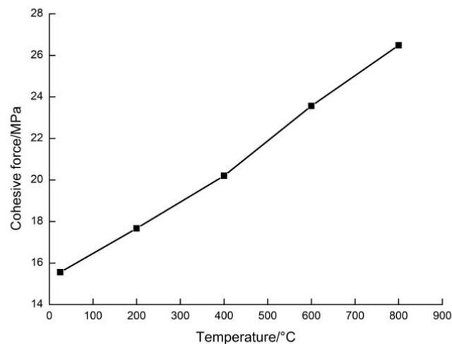
**Figure 9.** Relationship between sandstone cohesion and temperature.
