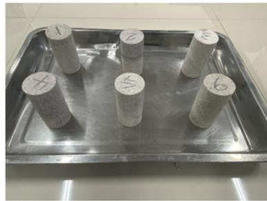
**Figure 2.** Sandstone specimens after high temperature treatment.
