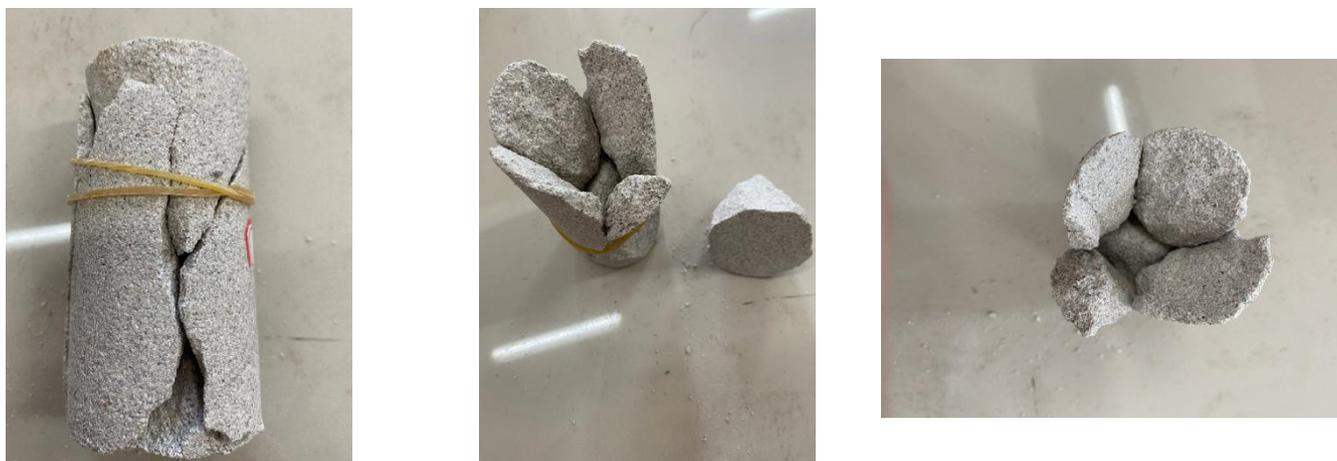
**Figure 10.** 600 °C sandstone specimens after damage.
