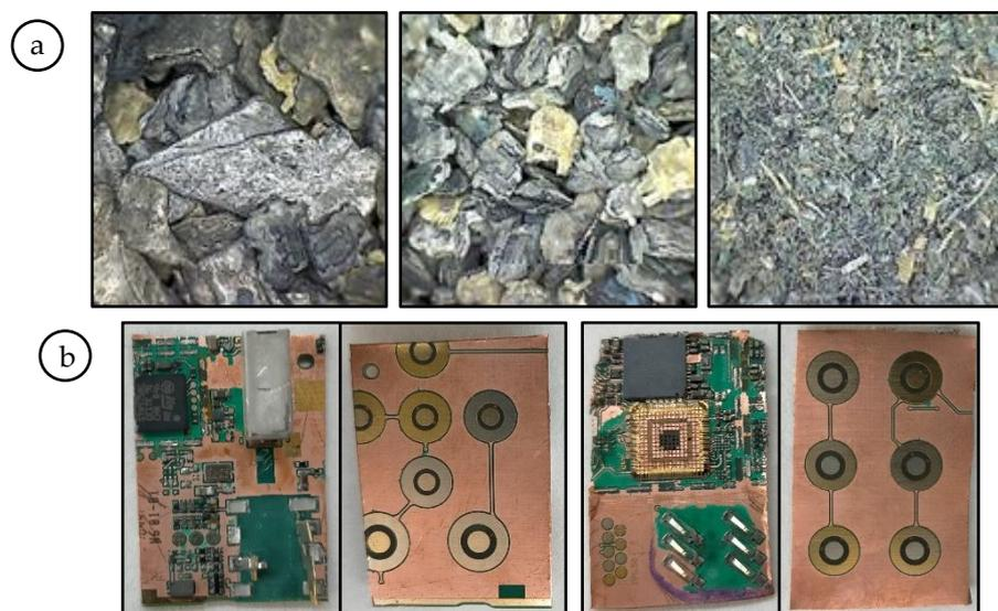
**Figure 2.** (a) Pulverized PCB sample according to particle size ( $>1.25 \text{ mm}$ ,  $1.25\text{--}0.75 \text{ mm}$  and  $<0.75 \text{ mm}$ ) (1:30 magnification) and (b) entire PCB pieces ( $3.5 \text{ cm} \pm 0.6 \text{ cm} \times 2.1 \text{ cm} \pm 0.1 \text{ cm}$ ) after treatment with a 10 M NaOH solution.
