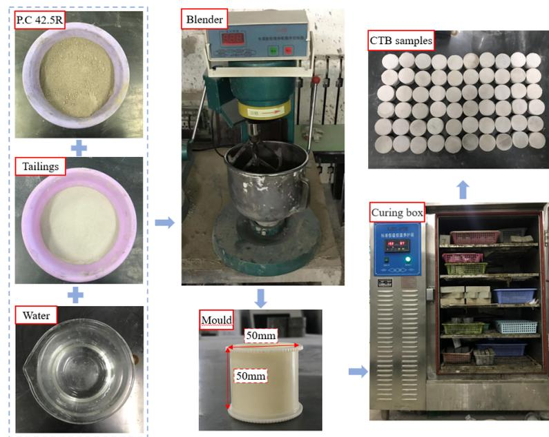
Figure 3. Preparation process of CTB specimens.
