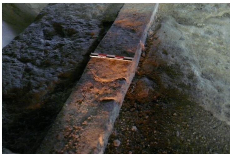
Figure 3. Welding line observed on TN3 tie-rod.
