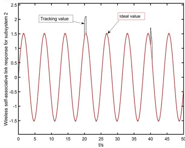
Figure 5. Wireless correlation failure mode for subsystem 2.
