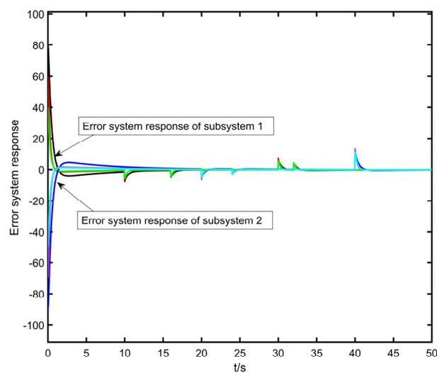
Figure 7. Overall tracking error system in subsystem 1 and subsystem 2 failure modes.
