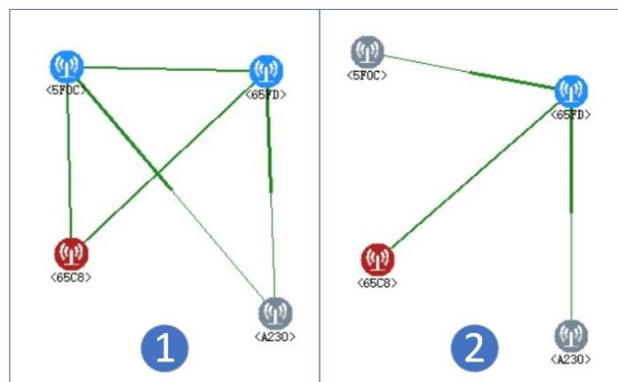
**Figure 9.** Wireless self-organizing network topology without adding the controller designed in this paper.
