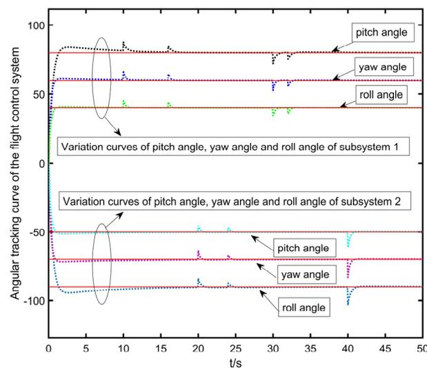
Figure 3. UAV subsystem flight control in failure mode.
