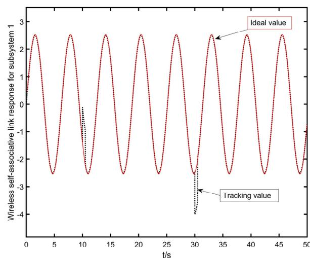
Figure 4. Wireless correlation failure mode for subsystem 1.
