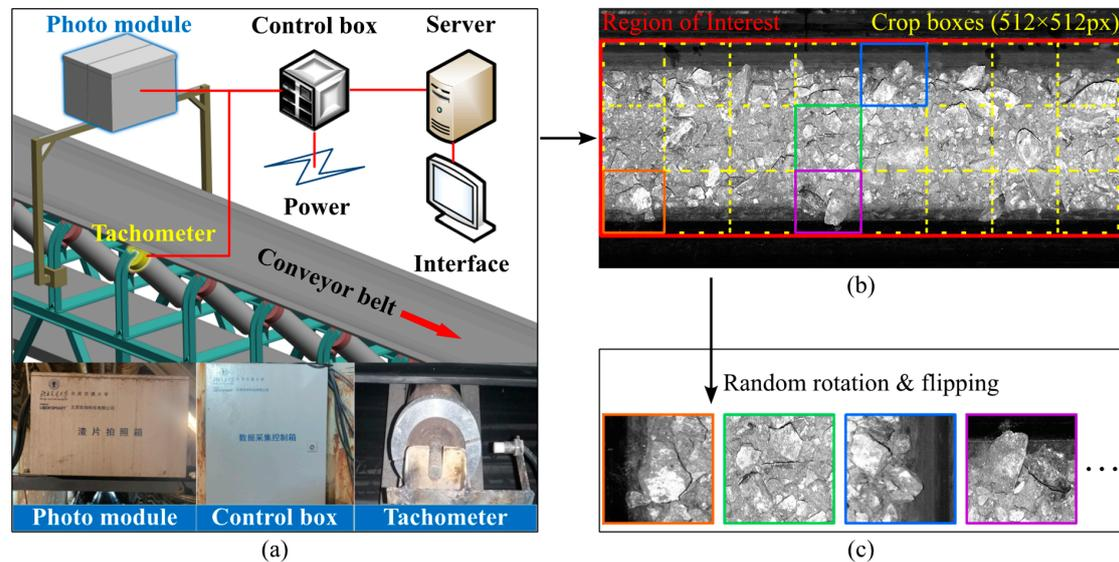
**Figure 11.** Data preparation procedure: (a) Image acquisition system; (b) ROI and crop boxes; (c) Training samples.
