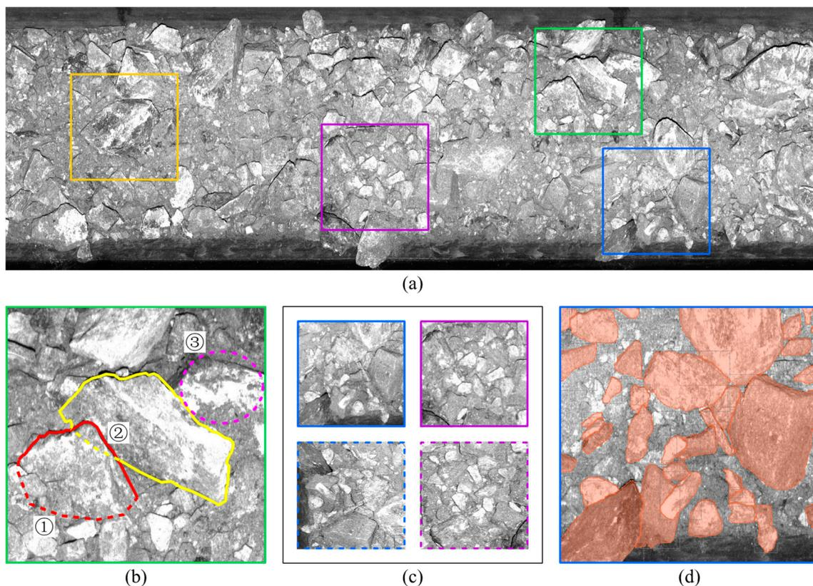
**Figure 1.** Characteristics of TBM muck image. (a) A sample muck image collected during TBM advancing. (b) The muck chips may present unfavorable characteristics such as the following: ① Invisible boundary; ② Overlapping; ③ Confusing texture. (c) The local image indicated by the blue and violet boxes, with the dashed boxes showing the results after rotation. (d) Muck chip annotations in blue box.
