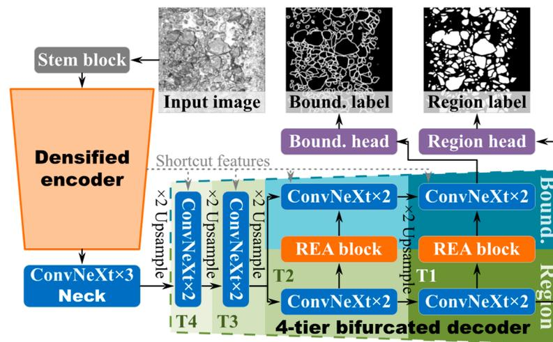
Figure 10. Structure of MuckSeg for formal segmentation task.
