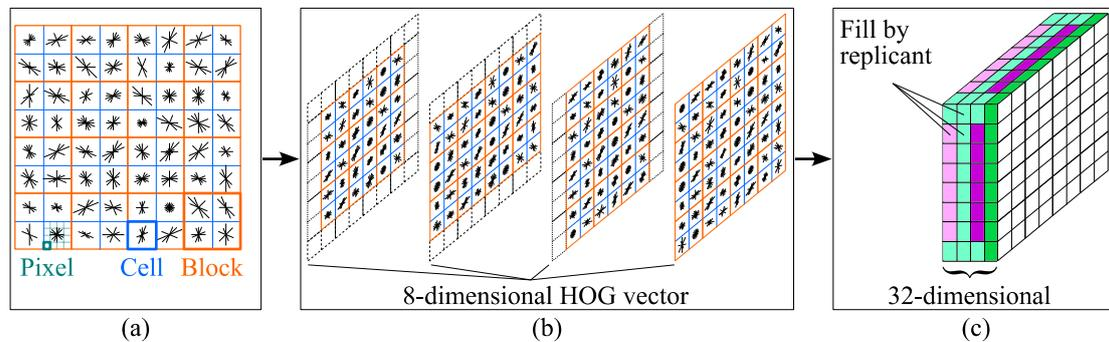
**Figure 5.** Schematic diagram of calculation steps for HOG descriptor. (a) Cell-wise HOG descriptor with 8 bins; (b) Block-wise normalization by sliding window; (c) Filling and concatenation.
