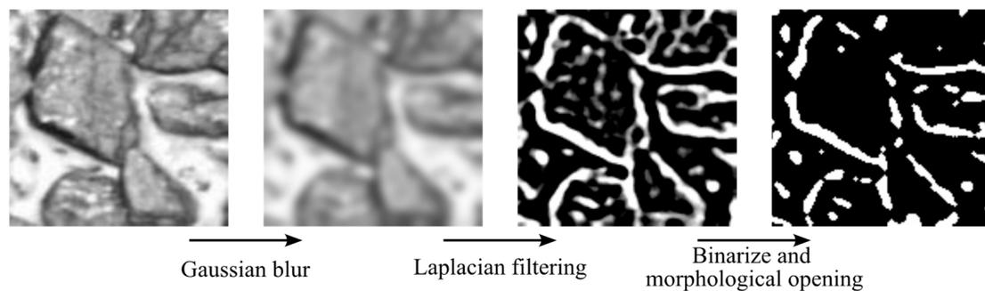
**Figure 6.** Schematic diagram of calculation steps for Laplacian feature.
