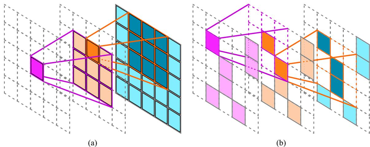
**Figure 3.** Schematic diagram of sparse convolution operator. (a) Dense convolution; (b) Sparse convolution.
