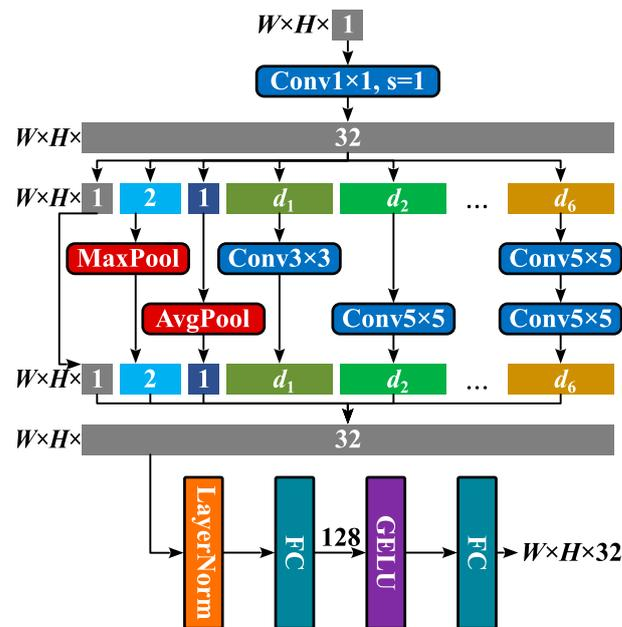
Figure 8. Structure of stem block in MuckSeg-SS-FCMAE.
