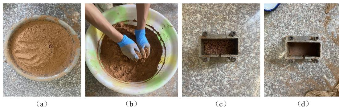
**Figure 11.** Preparation process of specimens. (a) Natural soil; (b) mixing soil; (c) before compacting; (d) after compacting.
