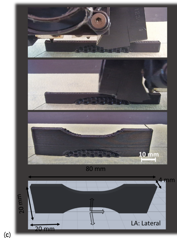
Figure 1. Ongoing 3D printing process of PLDA and three main orientations considered in this study: (a) vertical-VER, (b) horizontal-HOR, and (c) lateral-LAT.
