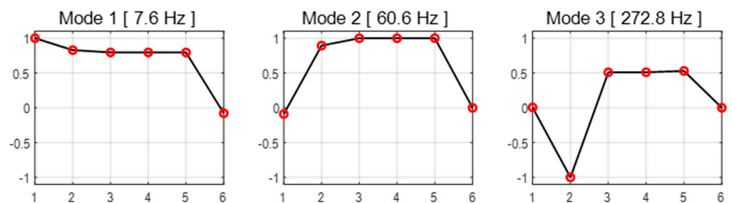
Figure 10. First three modes of the 6-DOF model.
