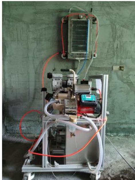
**Figure 4.** Second-generation wall impermeability testing instrument.
