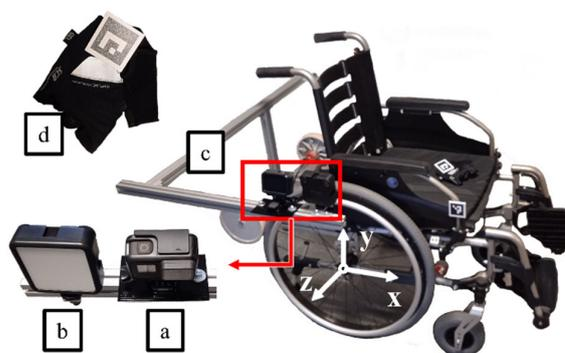
**Figure 1.** Measuring apparatus used in the research: (a) GoPro HERO 7 camera, (b) lamp, (c) boom, (d) Aruco marker.
