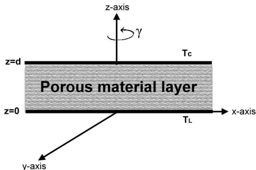
**Figure 1.** A rotating fluid saturated porous layer.
