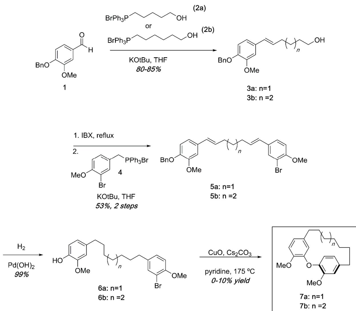
**Scheme 1.** Synthesis of diarylether cyclophanes of varying tether lengths. While small amounts of cyclophanes were obtained, low yields, high dilution, and complex reaction mixtures in the final step made this approach impractical.
