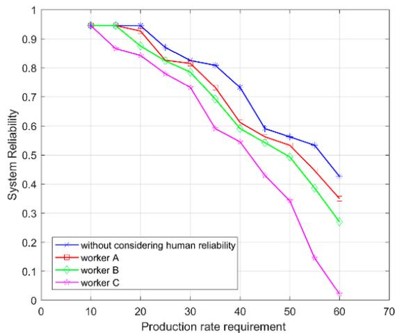
Figure 9. MSS reliability under different performance rate requirements.
