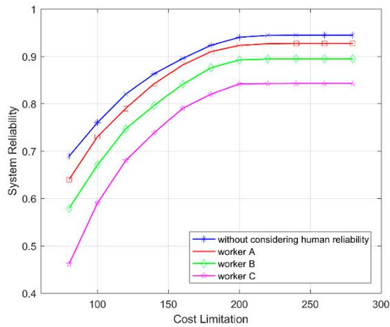
Figure 8. MSS reliability under different cost constraints.
