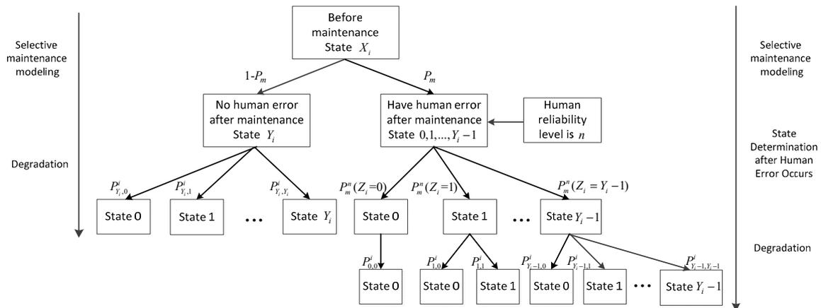
Figure 4. State change process of components.
