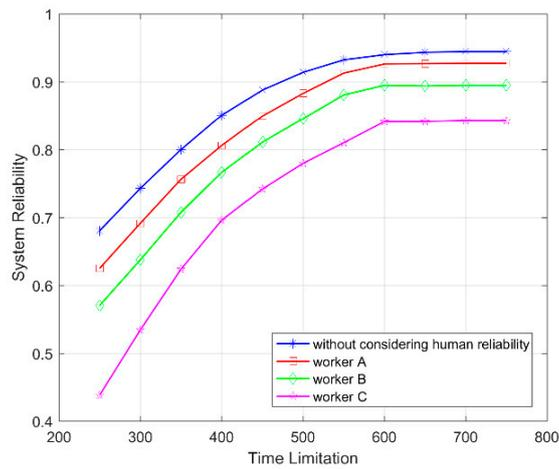
Figure 7. Multi-state system (MSS) reliability under different time constraints.
