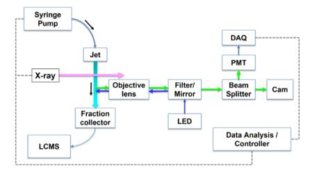
**Figure 6.** Conceptual diagram of inline dosimetry monitoring in XFMS experiments. Excitation light impinges on a flowing sample (capillary or jet delivery) immediately after X-ray exposure and before sample enters the fraction collector. The resulting fluorescence is collected along the same light path and analyzed to determine appropriate X-ray exposure values. Reproduced from [82], Figure 1A, used with permission.
