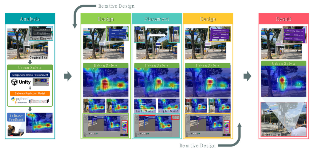
Figure 1. Incorporating saliency to iteratively enhance the conspicuity of a sign. Pedestrian attention is visualized throughout the design process, including site analysis, implementation, iteration, and installation. In this case, designers can simulate the amount of attention paid to wayfinding signs with different color and position (boxed elements in the mixed reality environment).
