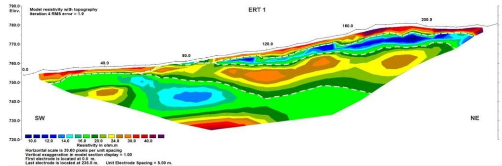
**Figure 10.** Electrical resistivity tomography (ERT 1) carried out parallel to the landslide body along the landslide foot. Dashed white lines outline possible sliding surfaces. Elev.: elevation above sea level.
