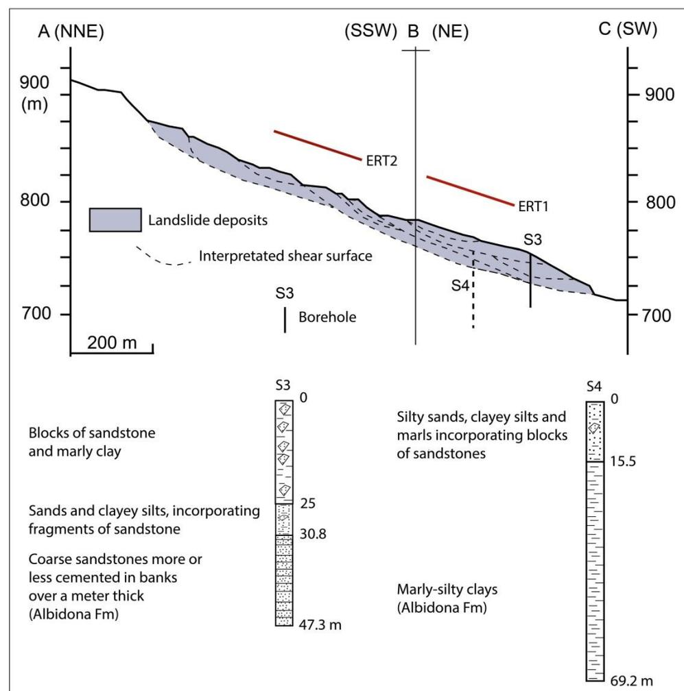
**Figure 8.** Geomorphological section of the Servigliano landslide of 1907 with superimposed boreholes according to Lentini & Schilirò (1982)<sup>3</sup>. For sections outline (A-B and B-C) see Figure 7. The Figure also shows the location of ERT (see Section 3.2.).
